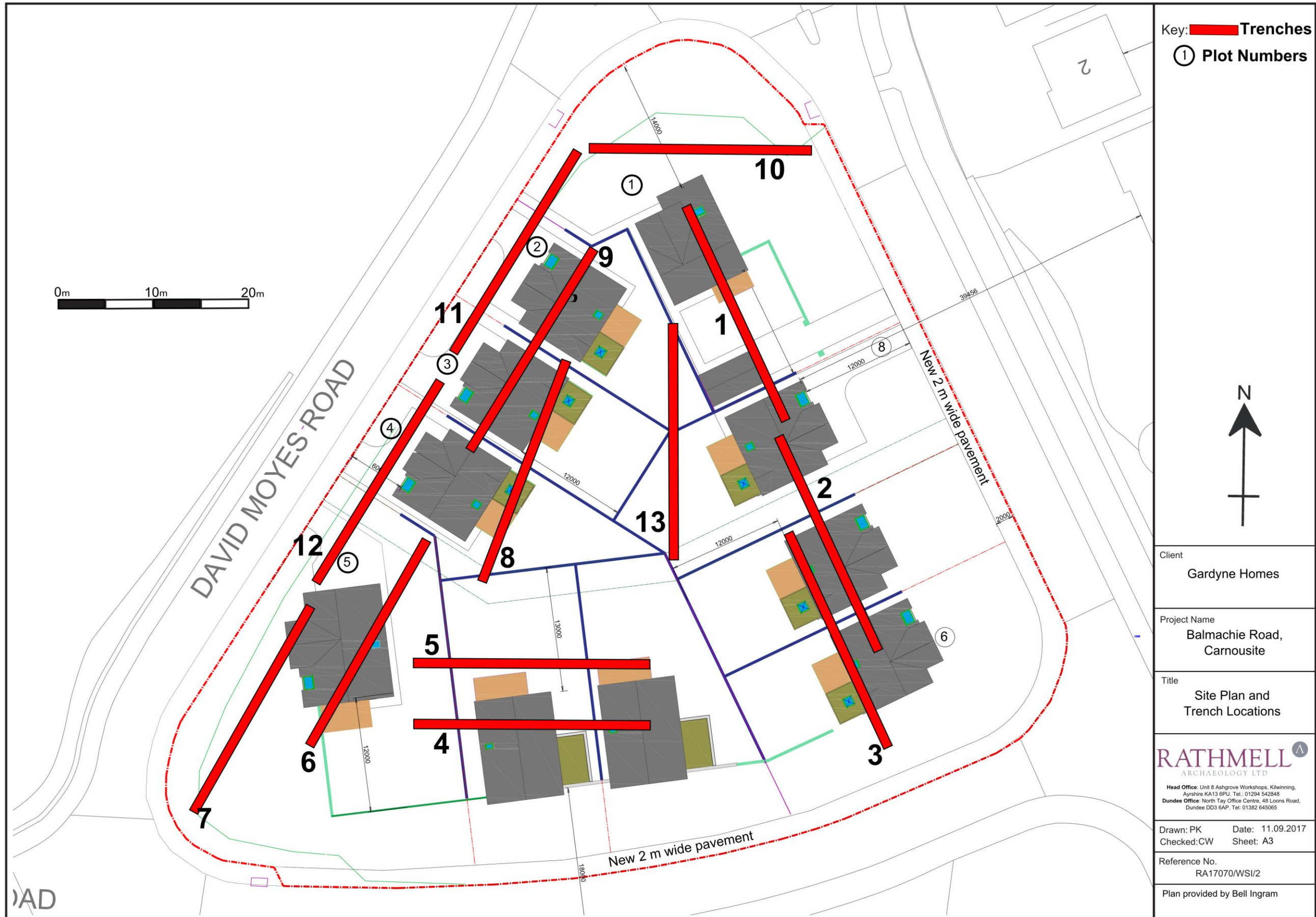
Figure 2: Plan of trenches as excavated.
