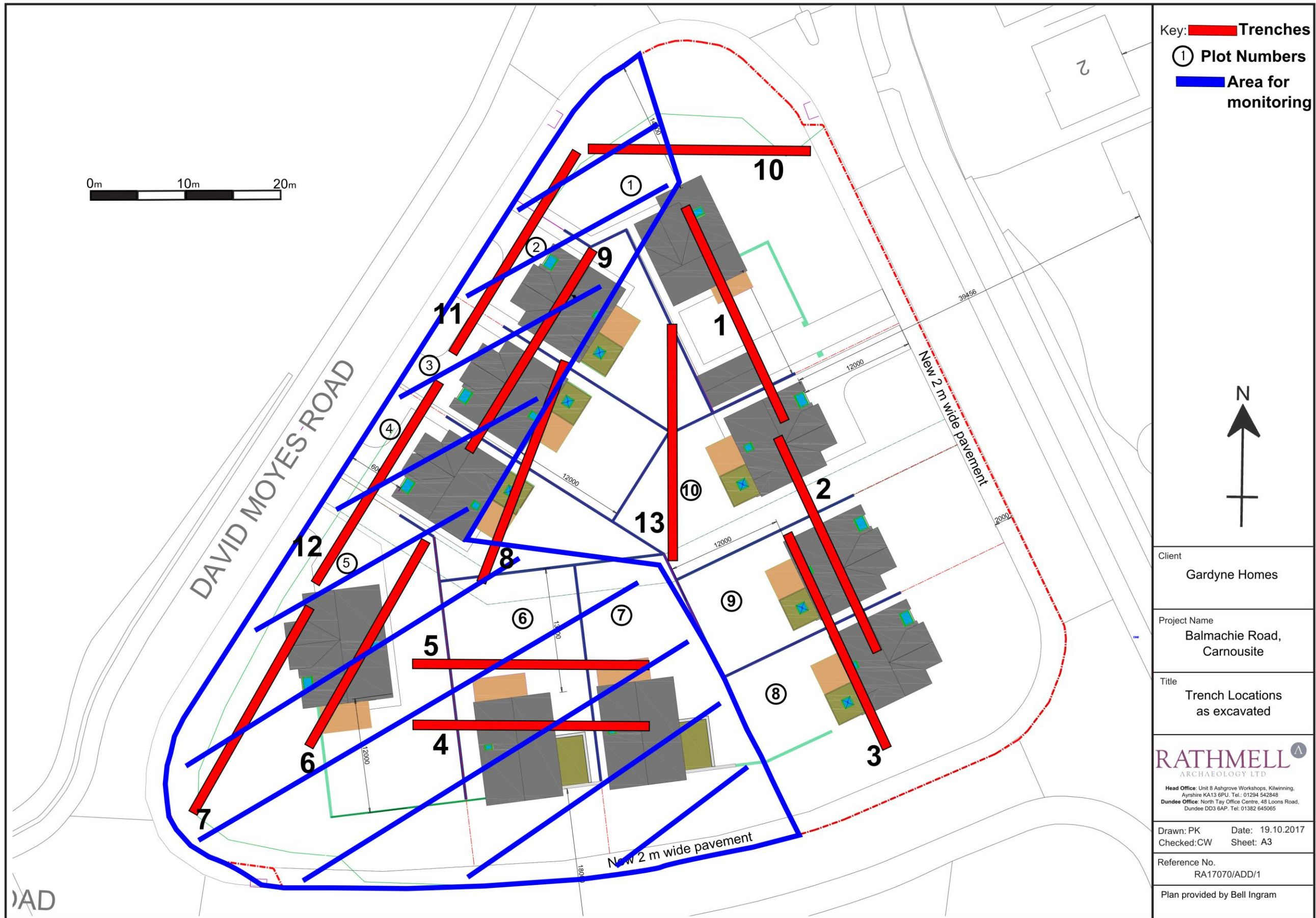
Figure 2: Plan of trenches as excavated and monitoring area (Planning Ref: 17/00450/FULL)
