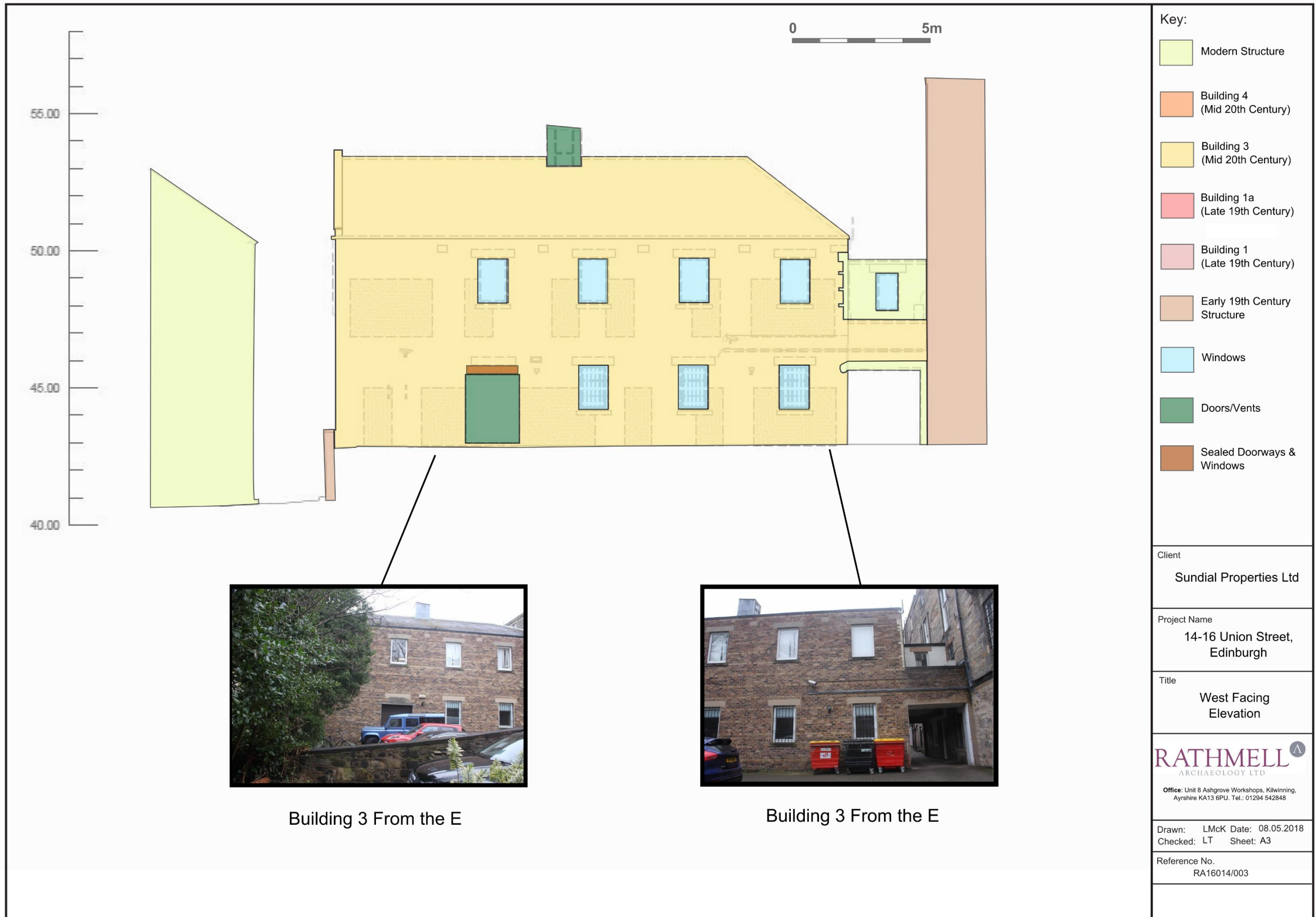
Figure 3: West facing elevation of Building 3, including the raised platform/roof and corridor.
