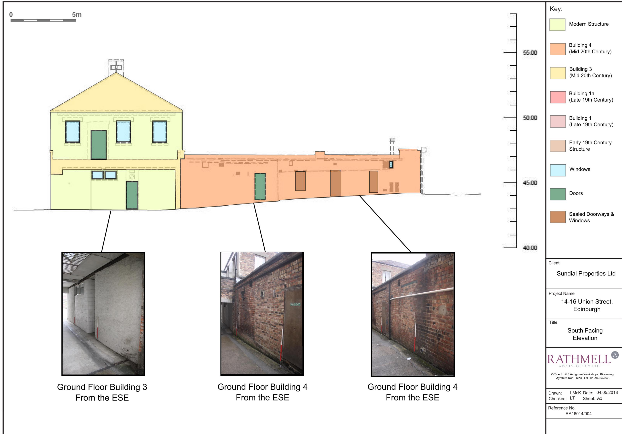
Figure 4: South facing elevation of Building 3 and 4.
