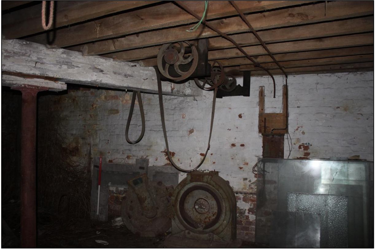
Figure 14a: Room C - Ceiling-mounted Drive Shaft and Dismantled Drum from Grain Bruiser
