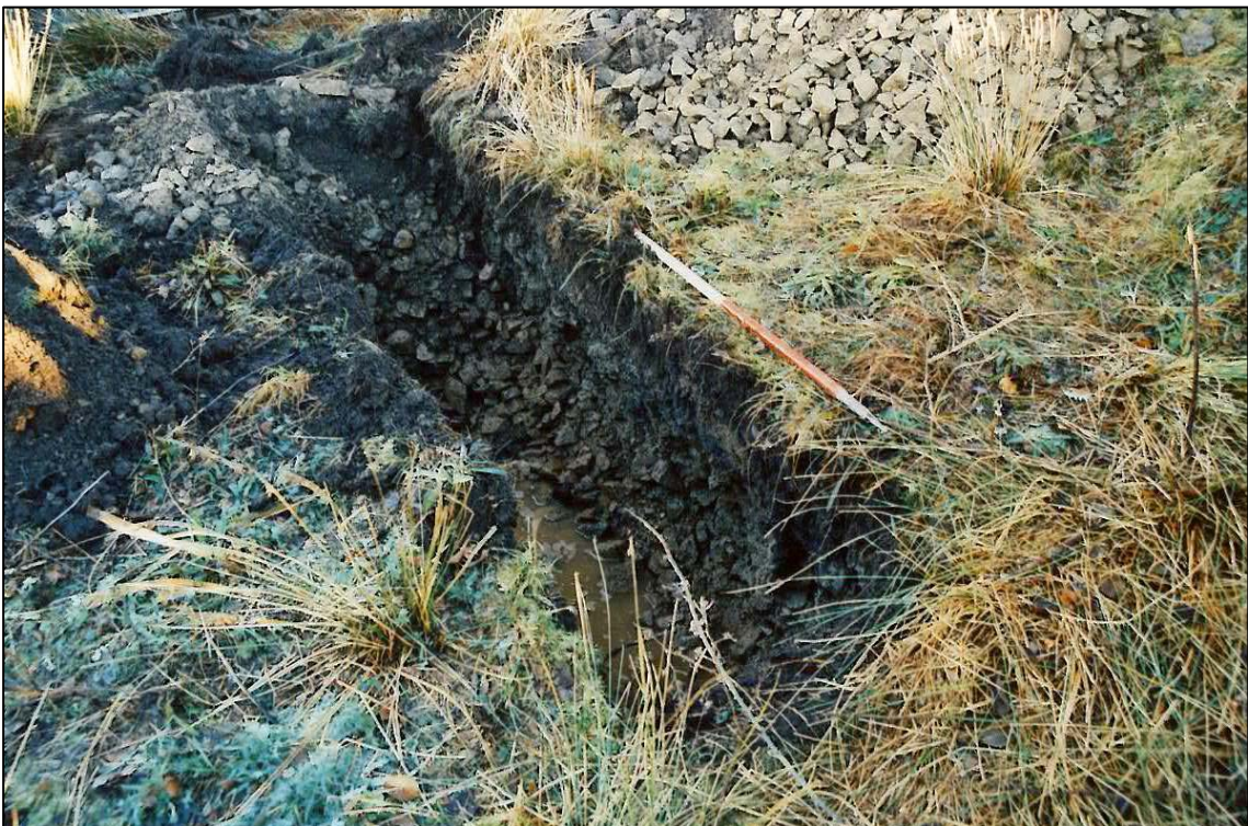
Figure 4b: Test Pit 3, note engineered material at depth
