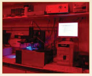
Analysing OSL samples in the lab: A TL/OSL DA-15 Risø reader equipped with blue LEDs in the Luminescence Dating Laboratory, University of Oxford (Photo © Jean-Luc Schwenninger)
