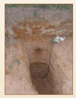
OSl field technique: a gamma spectrometer measuring the natural radiation present in a Quaternary sediment
