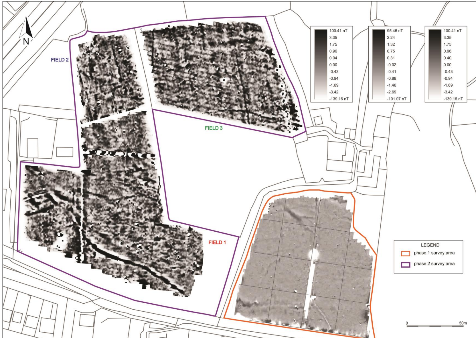
SHADE PLOT OF GRADIOMETER SURVEY DATA; BAND WEIGHT EQUALISED; GRADIATED SHADING.
