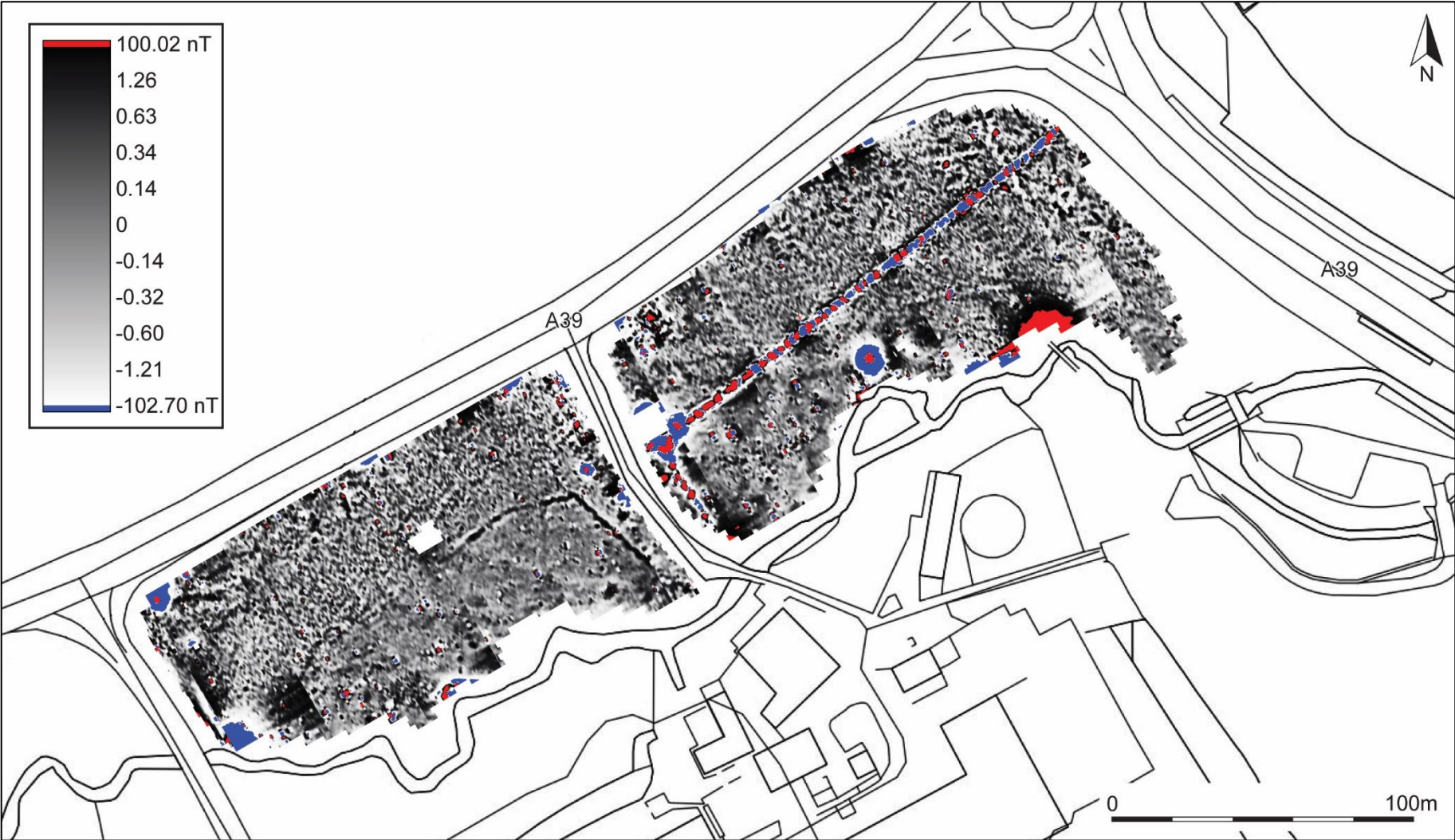
FIGURE 6: RED-GREY-BLUE SHADE PLOT OF GRADIOMETER SURVEY DATA; BAND WEIGHT EQUALISED; GRADIATED SHADING.
