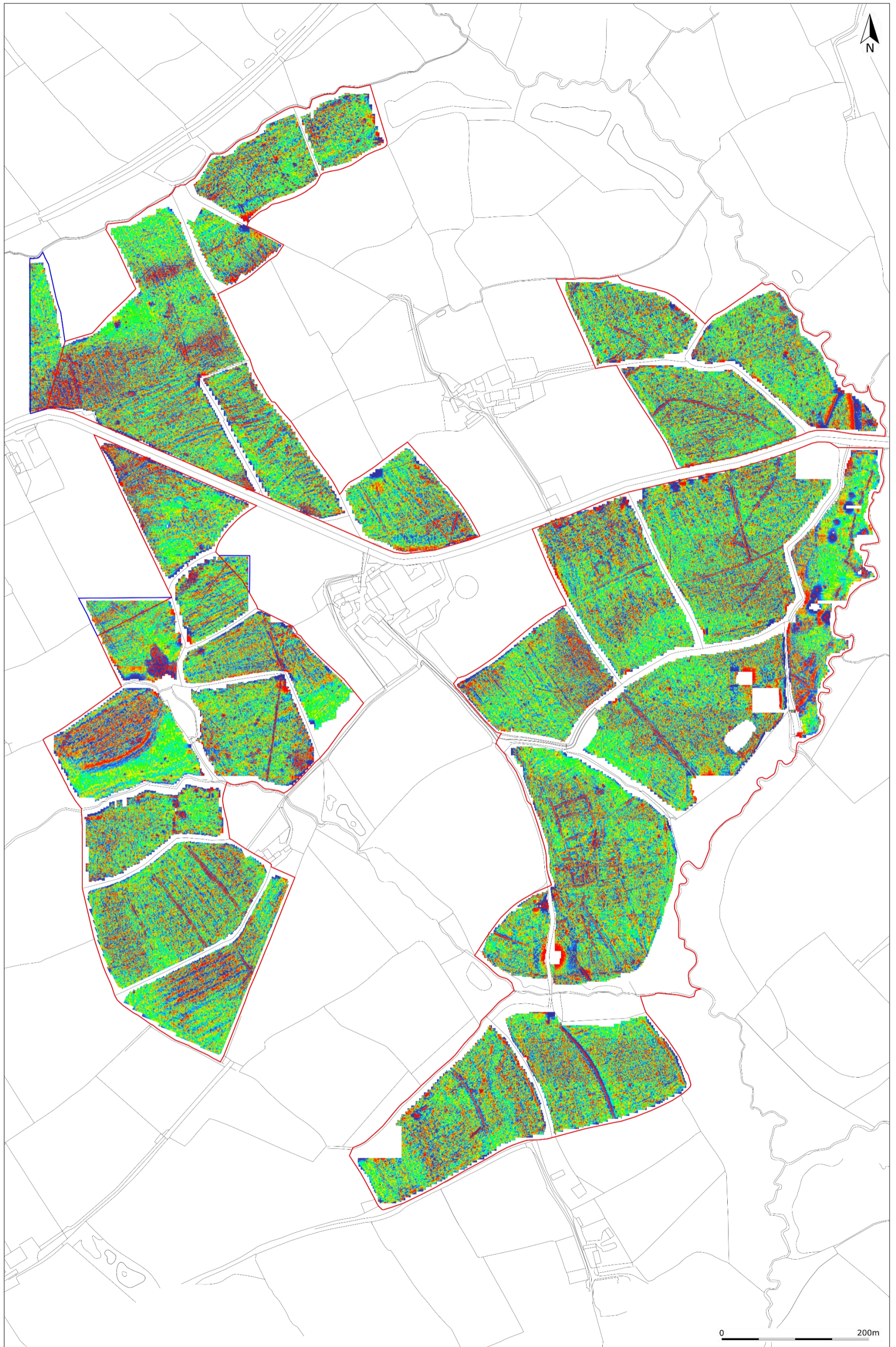
8. RED-GREEN-BLUE 2 SHADE PLOT OF THE GRADIOMETER SURVEY DATA; BAND WEIGHT EQUALIZED; GRADIATED SHADING.
