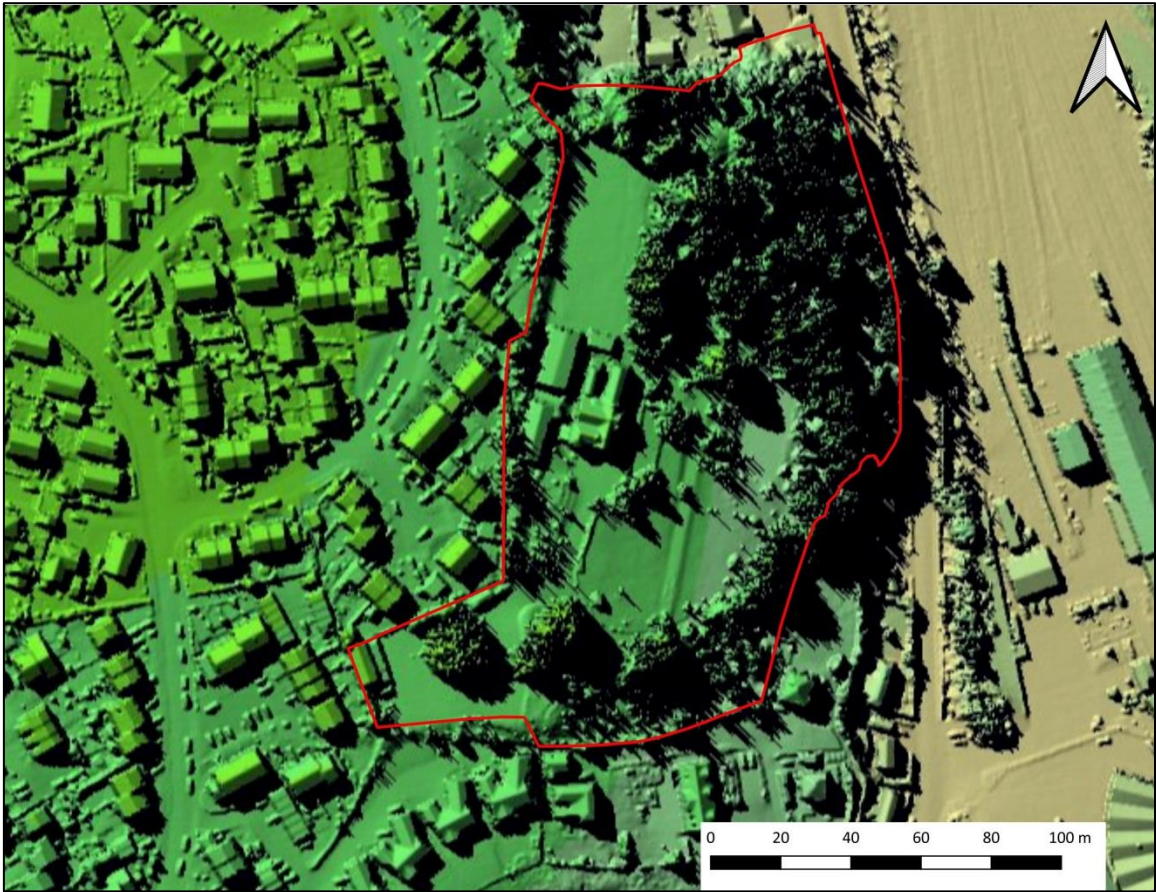
FIGURE 8: LIDAR 50CM DSM DATA PROCESSED BY THE ENVIRONMENT AGENCY. THE APPROXIMATE STUDY AREA IS INDICATED. CONTAINS PUBLIC SECTOR INFORMATION LICENCED UNDER THE OPEN GOVERNMENT LICENCE.
