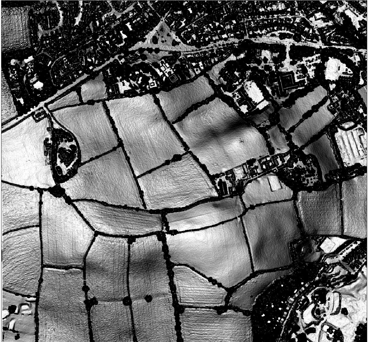
Figure 21: QGIS image (terrain analysis>slope) of LiDAR survey data [contains freely available LiDAR data supplied by Natural Environment Research Council (Centre for Ecology & Hydrology; British Antarctic Survey; British Geological Survey); ©NERC (Centre for Ecology & Hydrology; British Antarctic Survey; British Geological Survey)].
