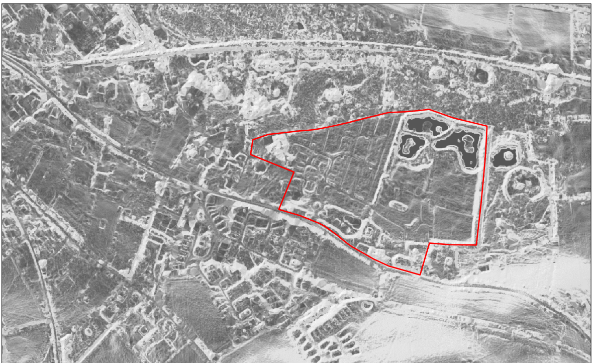
FIGURE 10: 1M DTM LIDAR SLOPE IMAGE DATA PROCESSED USING QGIS 3.12 MULTIHILLSHADE. THE SITE BOUNDARY IS INDICATED. CONTAINS PUBLIC SECTOR INFORMATION LICENCED UNDER THE OPEN GOVERNMENT LICENCE.
