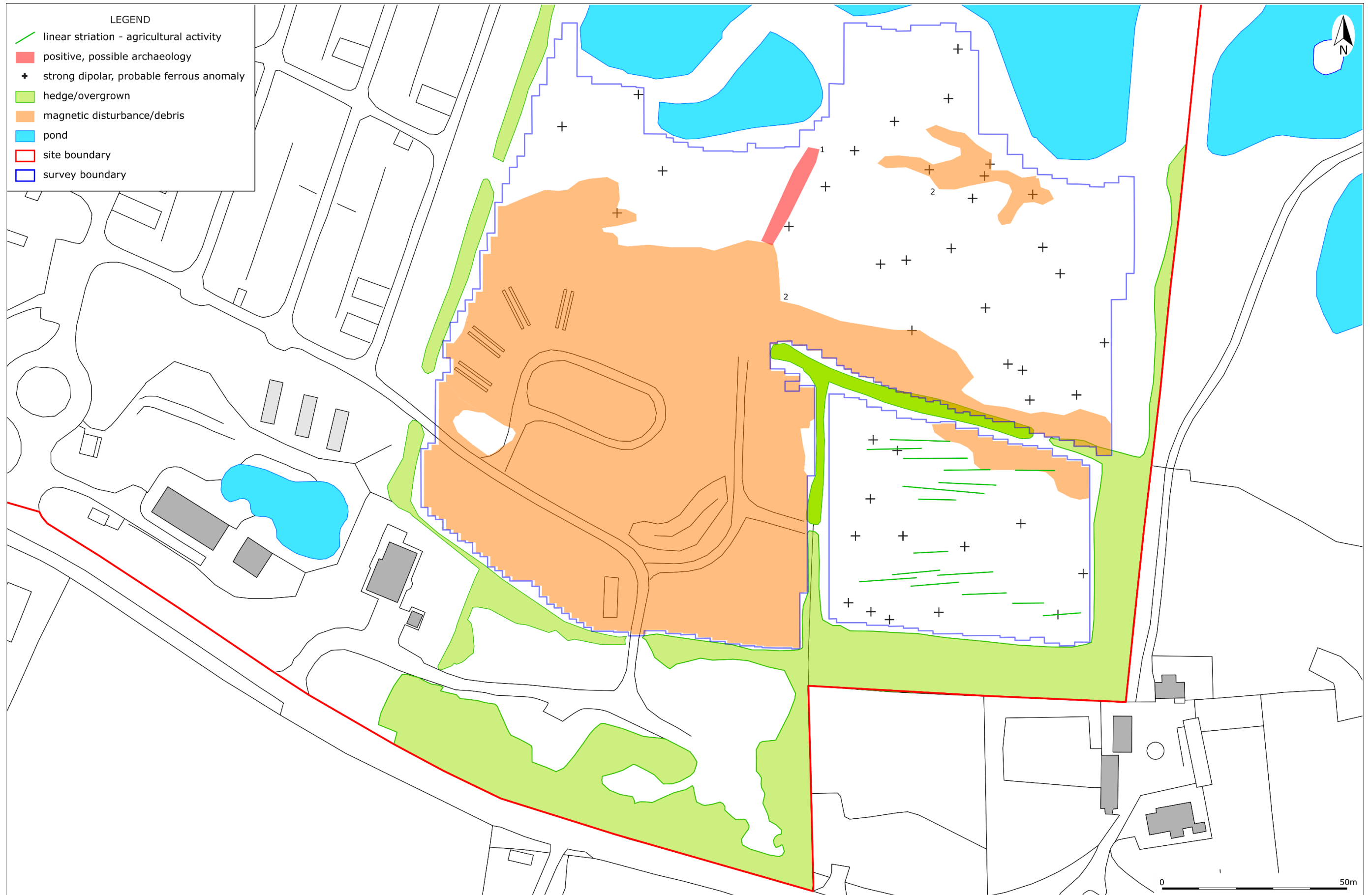
FIGURE 15: INTERPRETATION OF GRADIOMETER SURVEY DATA.
