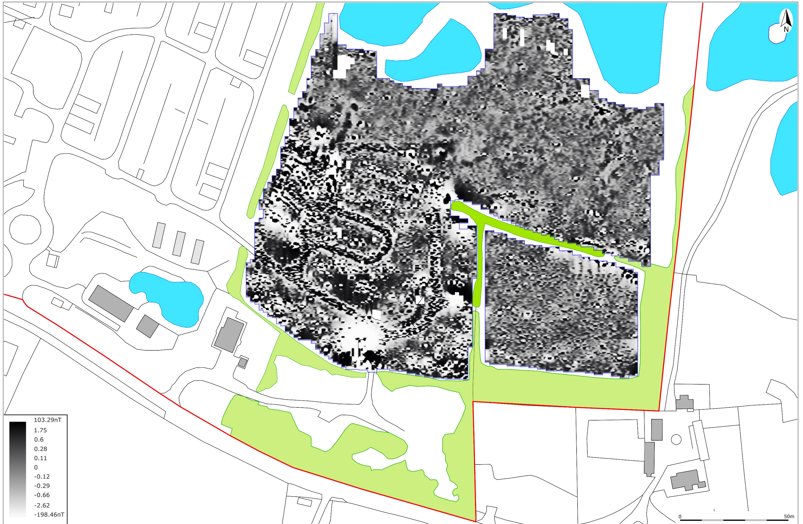
2. GREYSKALE SHADE PLOT OF GRADIOMETER SURVEY DATA; BAND WEIGHT EQUALIZED; GRADIATED SHADING.
