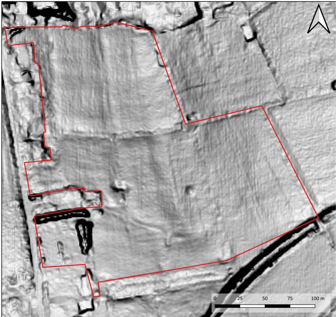
FIGURE 9: LIDAR 1M DTM DATA PROCESSED USING QGIS 3.16 SLOPE Z2. THE APPROXIMATE SITE BOUNDARY IS INDICATED. CONTAINS PUBLIC SECTOR INFORMATION LICENCED UNDER THE OPEN GOVERNMENT LICENCE.
