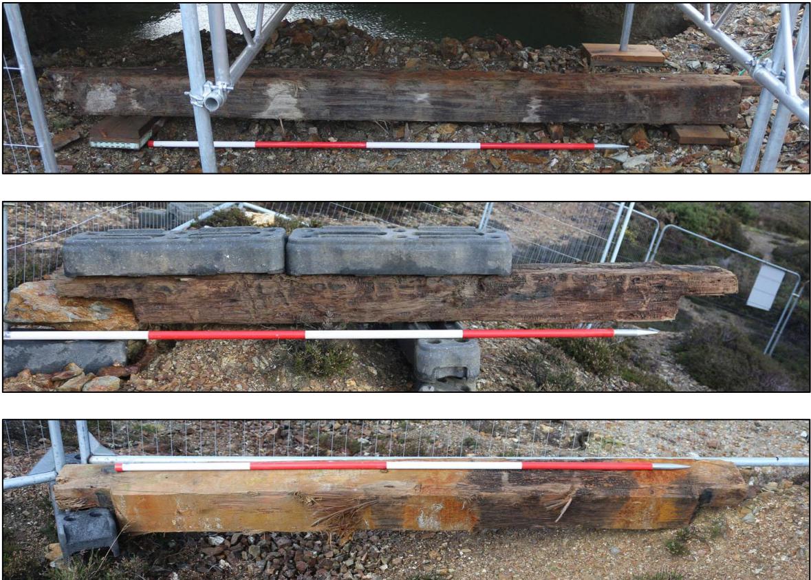
FIGURE 10: THE THREE TIMBERS RECOVERED FROM THE SHAFT CAPPING (2M SCALES).
