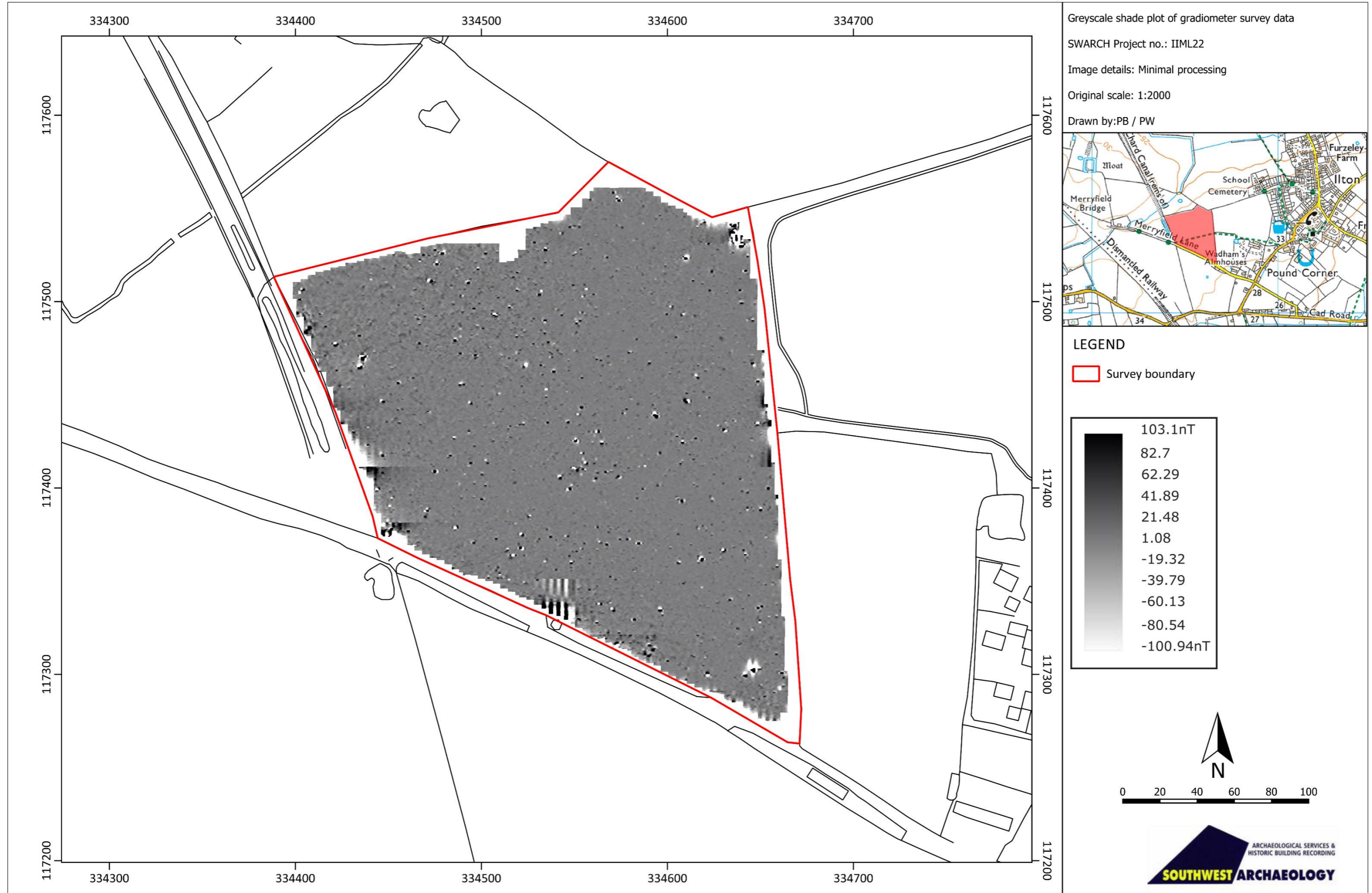
FIGURE 14: GREYSCALE SHADE PLOT OF THE GRADIOMETER SURVEY DATA; MINIMAL PROCESSING.
