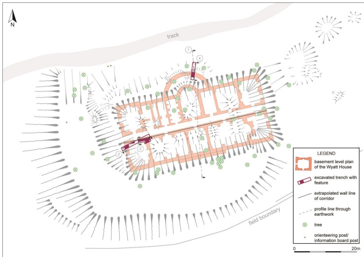
FIGURE 90: TRENCH AND FEATURE LOCATIONS AND LOCATED BASEMENT LEVEL PLAN OF THE WYATT HOUSE, C.1776, OVERLAYING THE EARTHWORK SURVEY (FROM SWARCH 2017, FIG.7).
