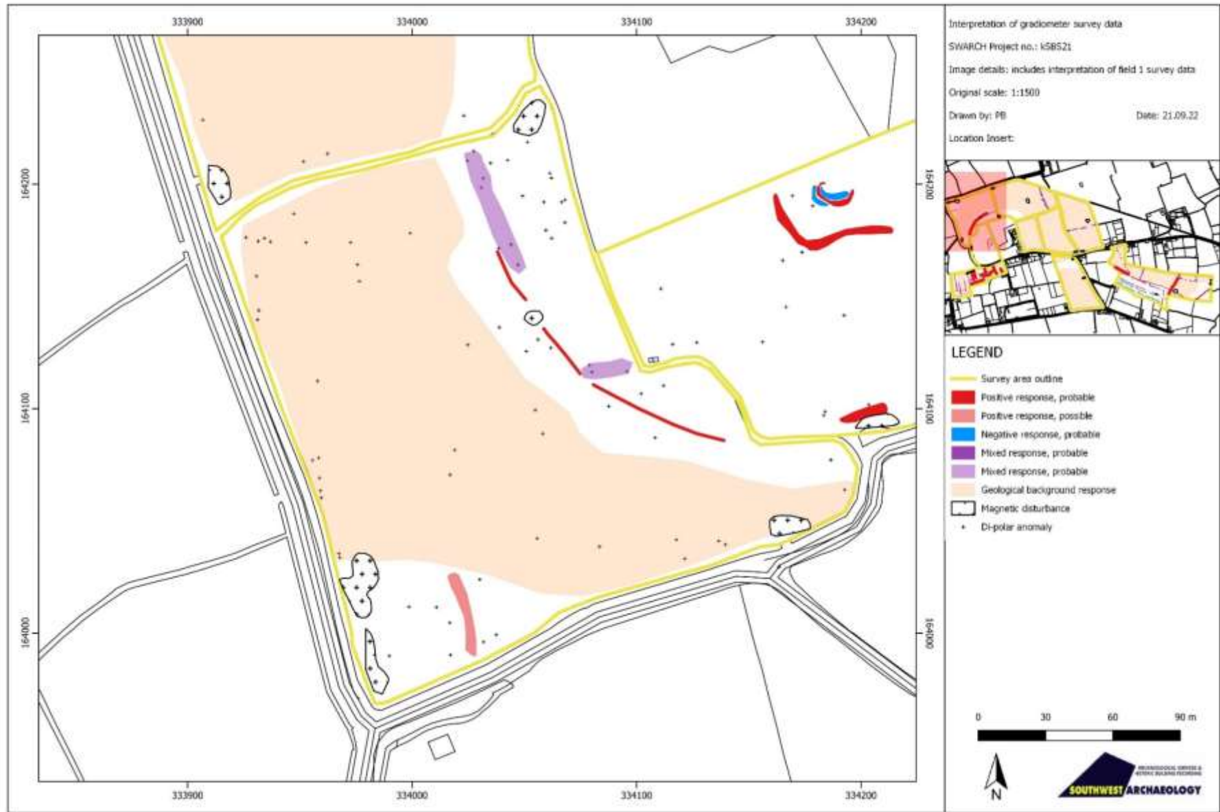
FIGURE 32: FIELD F1. INTERPRETATION OF GRADIOMETER SURVEY DATA.
