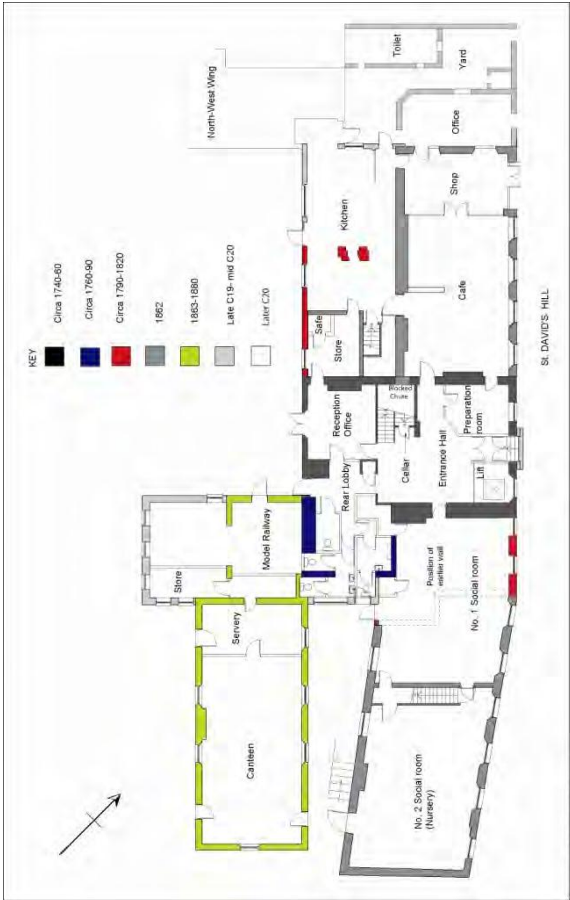
Phasing of Ground Floor
