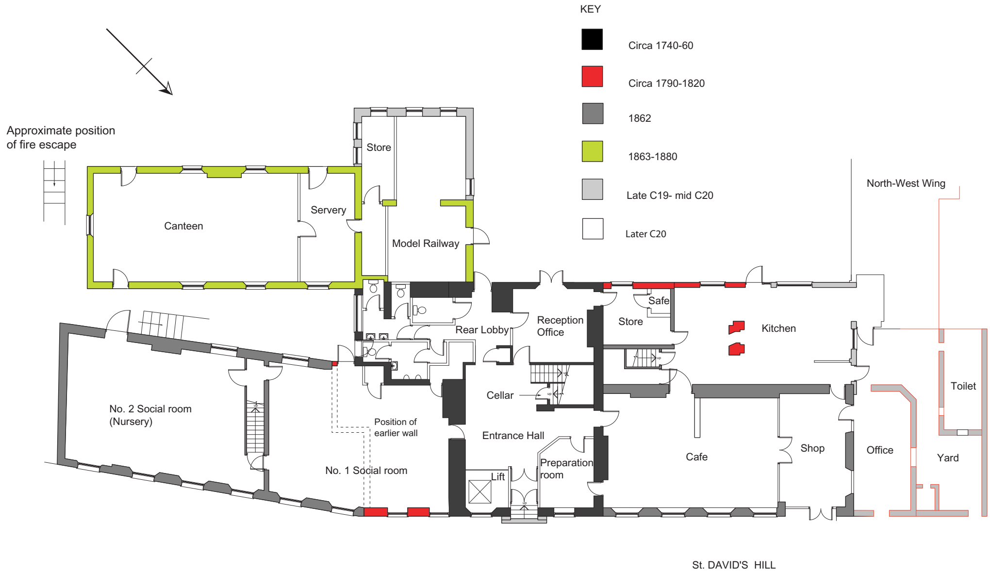
Fig 3: Community Centre, ground floor plan showing historic phasing, based on drawing supplied by King Sturge (Bristol), areas outlined in red, Not to scale.
