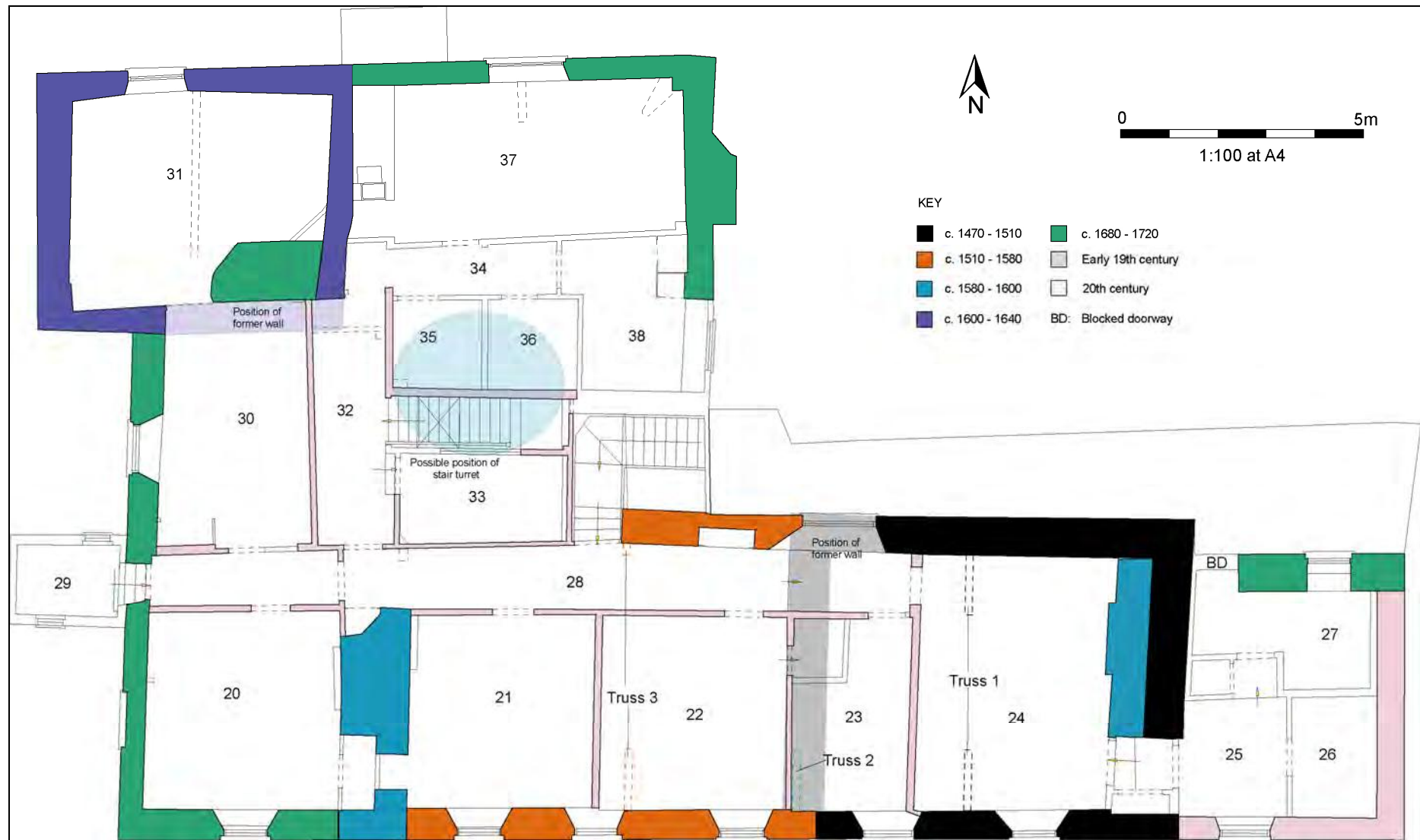
Figure 15: Phased plan of the first floor.
