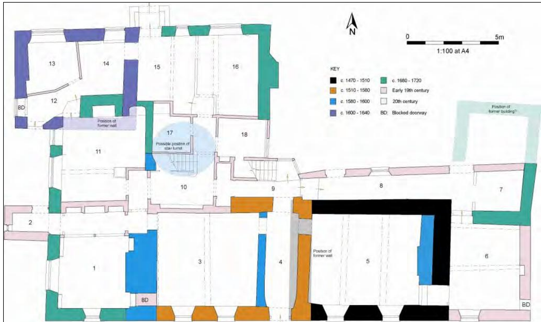
Figure 14: Phased plan of the ground floor.
