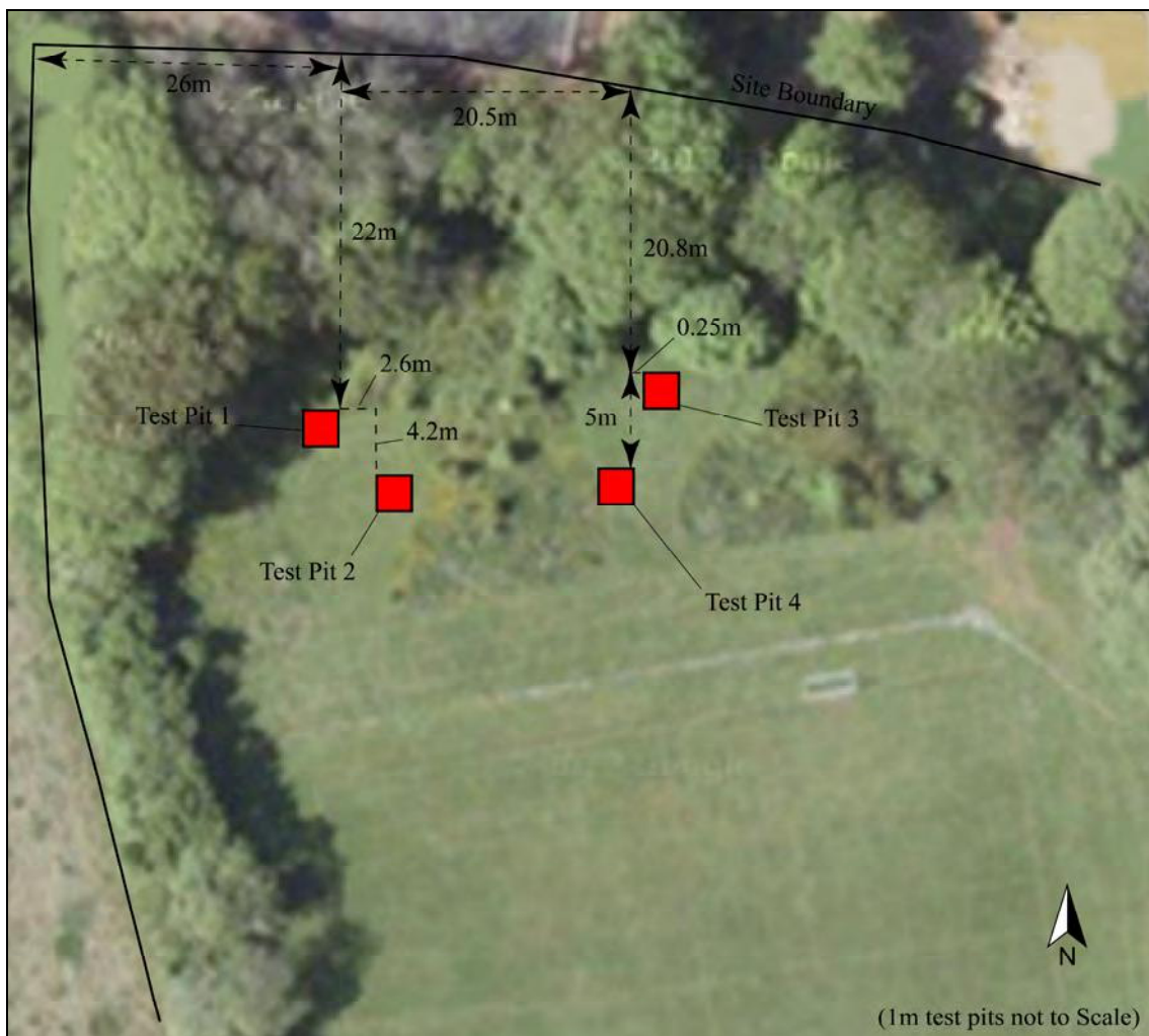
Figure 2: Measured location of 1m test pits from the north-east corner of the site boundary.
