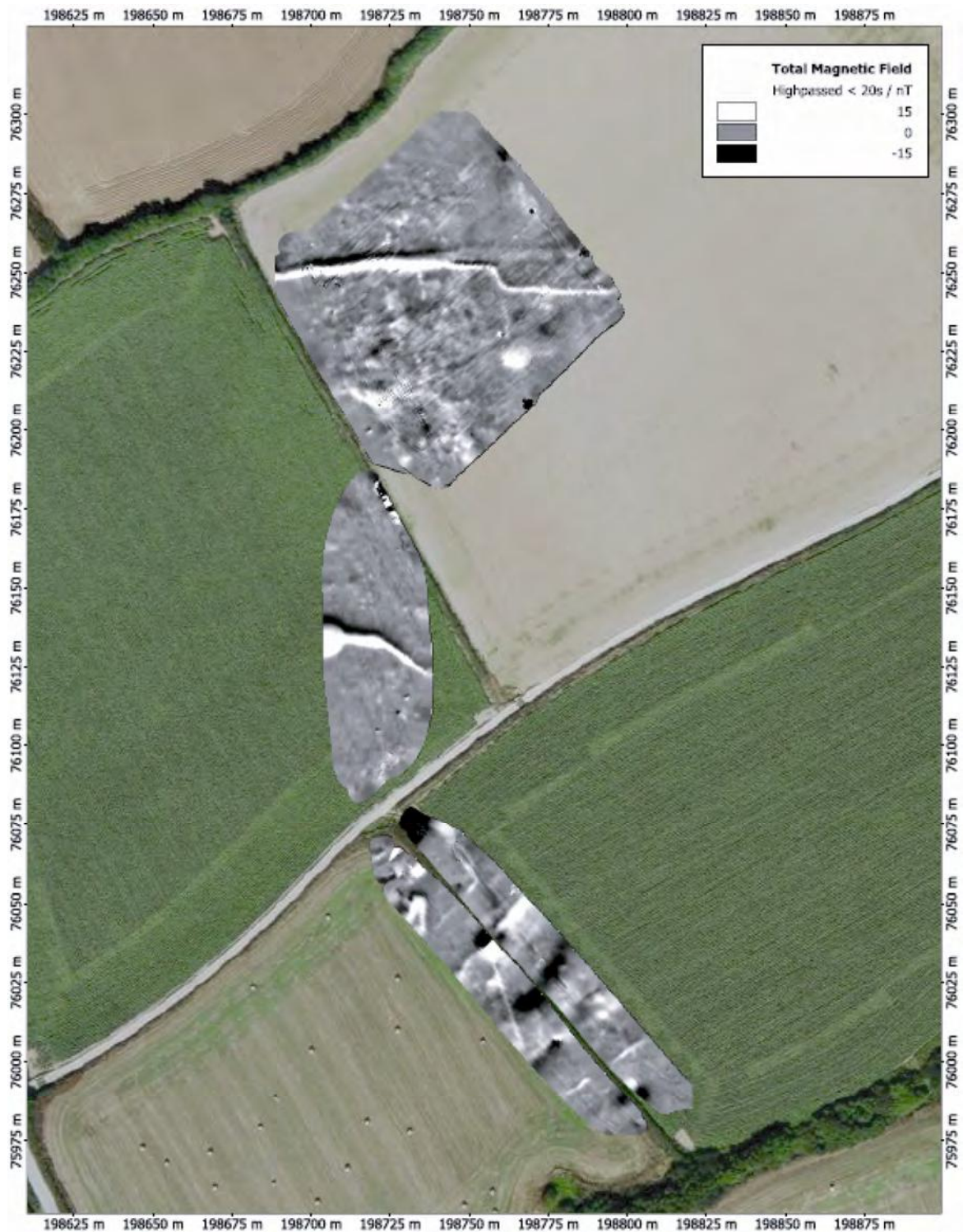
Figure 6: The results of the magnetometry (non-gradiometric (vertical) configuration) survey (source: ArchaeoPhysica).
