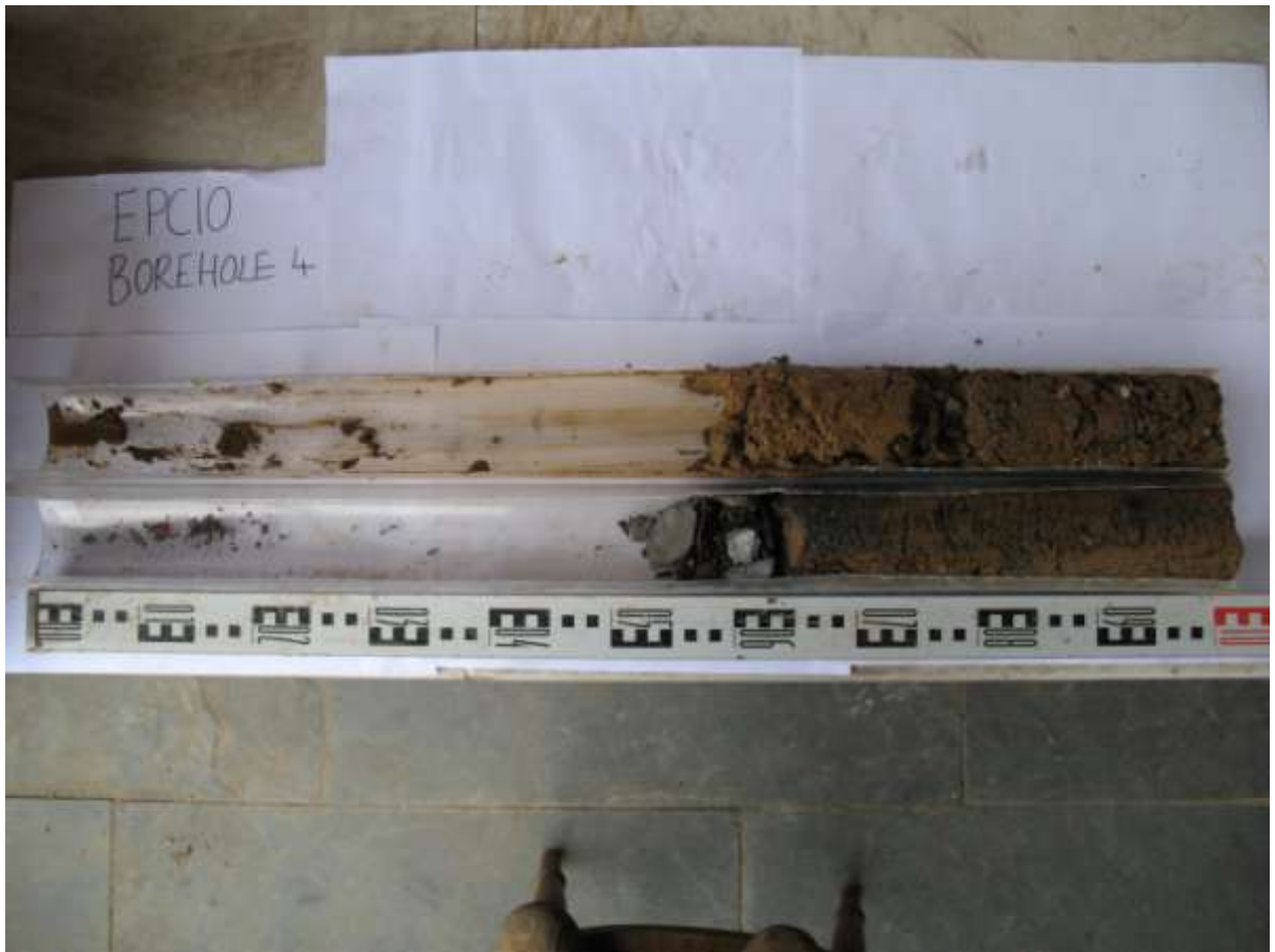
Figure 14: The cores from Borehole #4.
