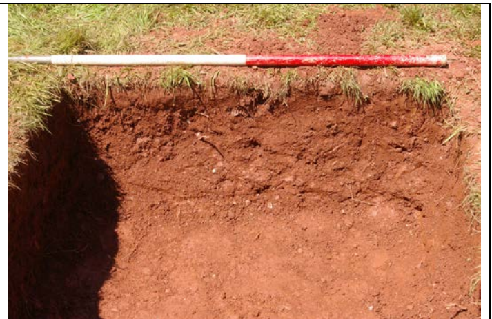
Figure 3: Test Pit 7 South Facing Section (1m scale).
