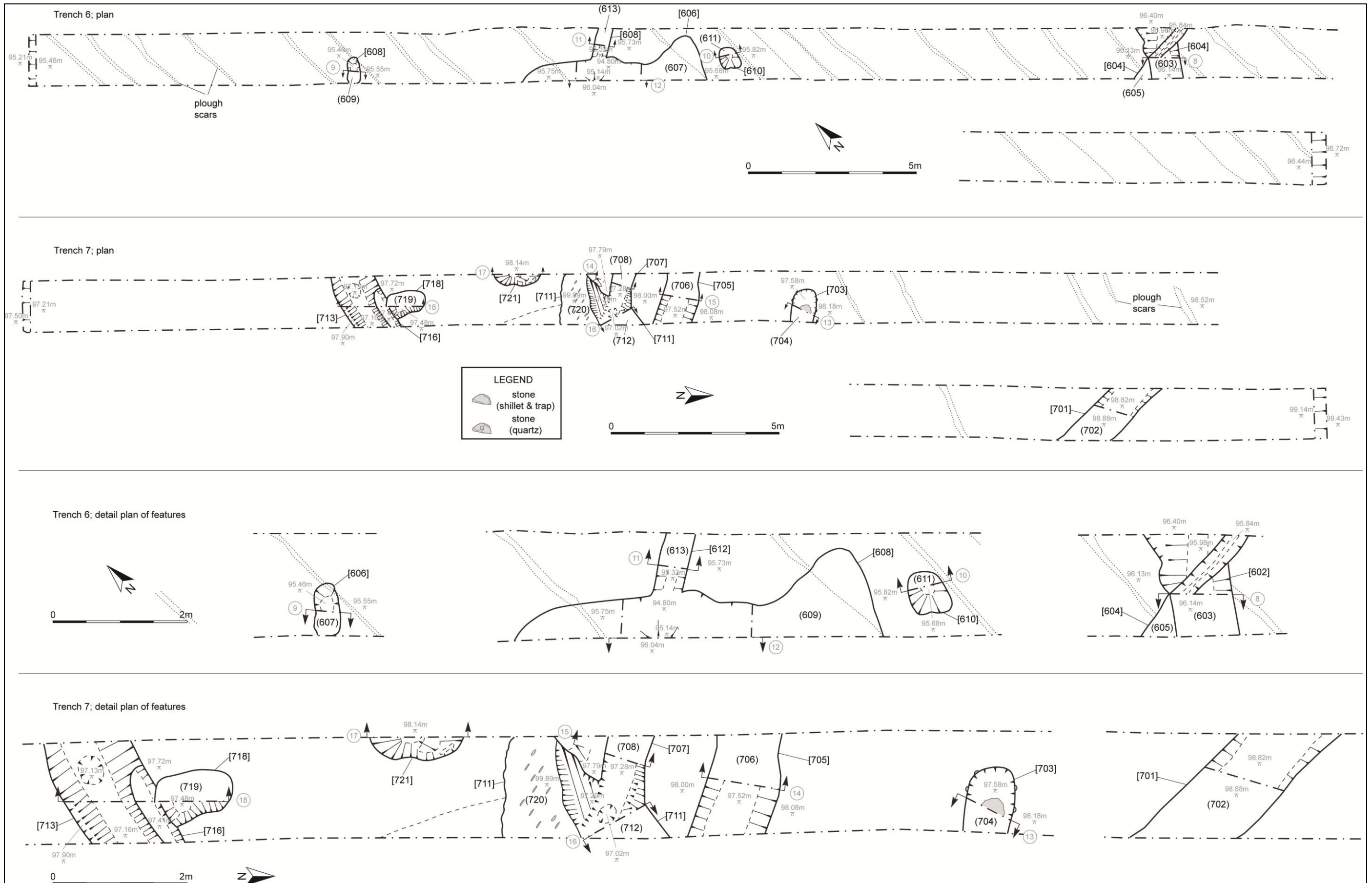
Figure 21: Plan for Trenches 6 and 7 including section numbers and larger scaled plans of features (n.b. levels of features from Trenches 6 & 7 calculated in relation to an arbitrary TBM of 100.00m AOD).
