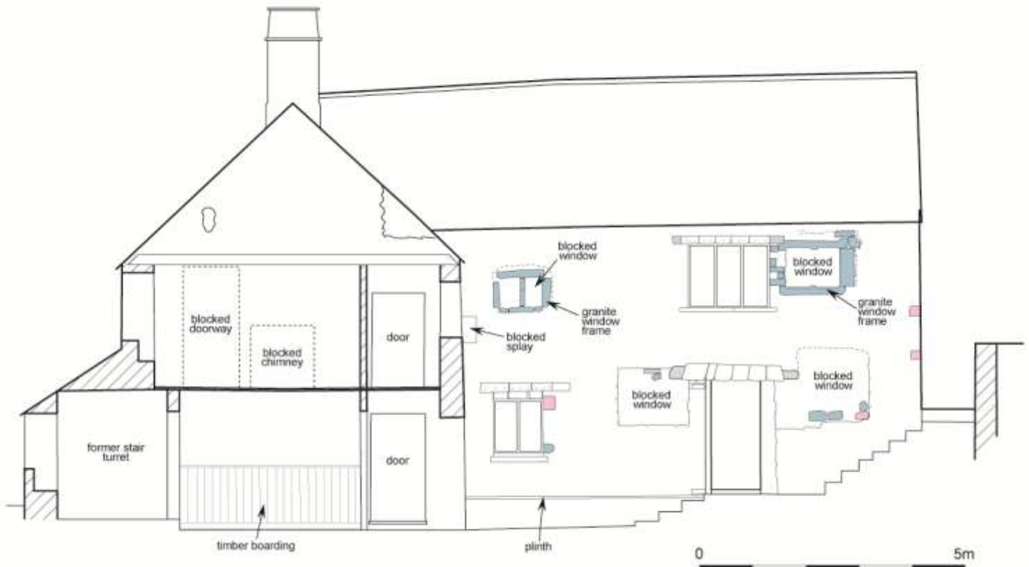
Figure 26: The north-facing elevation of the 15 th century block. Conventions: timber in grey; granite in blue; hard pinkish-red sandstone in pink.
