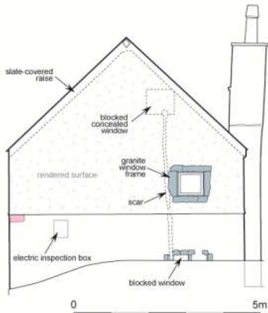
Figure 27: The west-facing gable of the 15 th century block.
