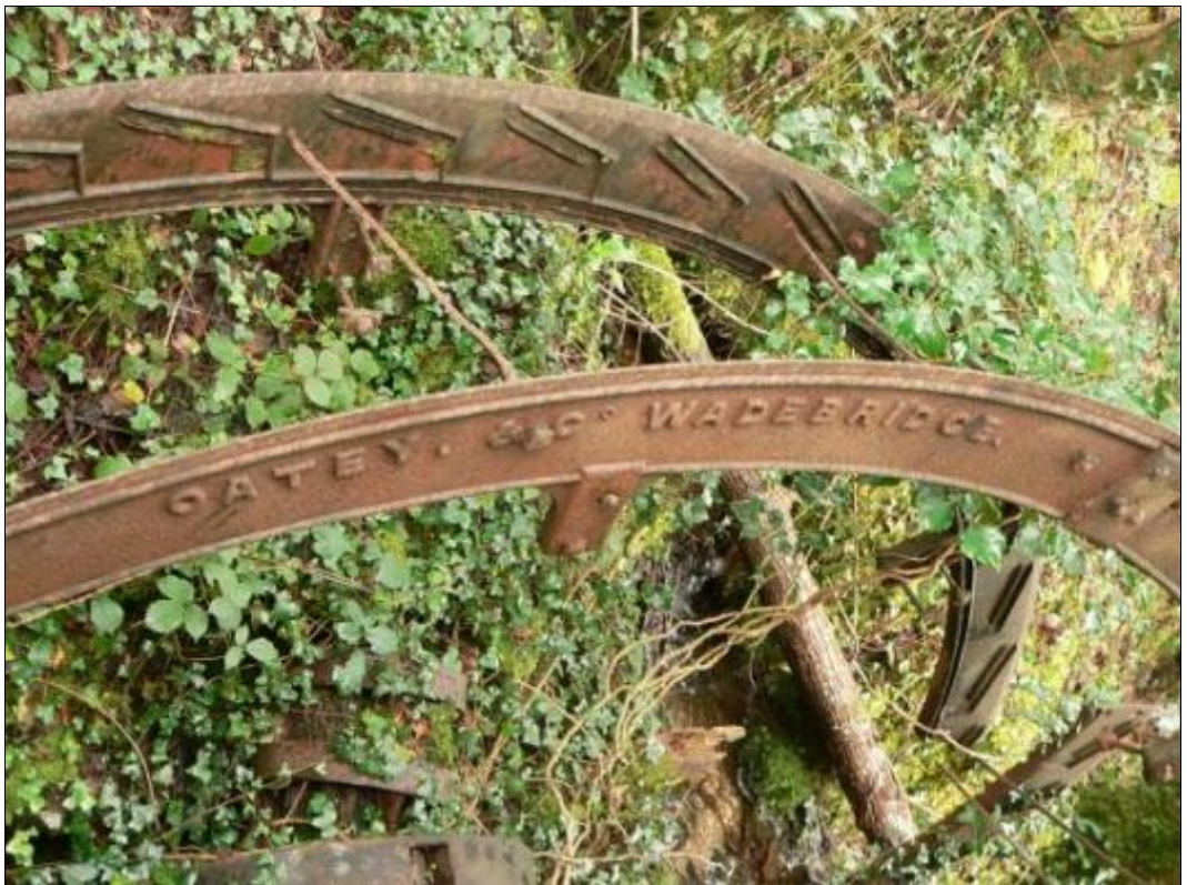
Waterwheel shrouds showing maker's name inscription.
