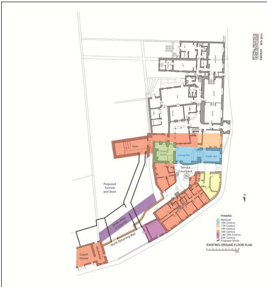
Figure 6: Plan of the building complex, showing the developmental phasing and proposed plans.
