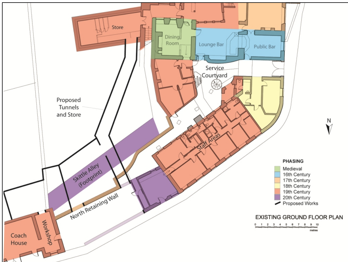
Figure 1: Phased plan showing the existing ground floor and proposed tunnels. Note the Skittle Alley is at first floor level.
