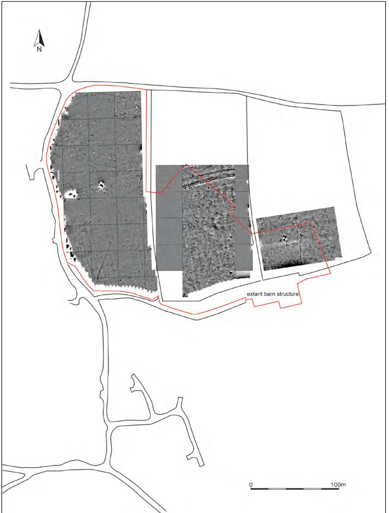
Figure 6: Shade plot of gradiometer survey results (the proposed site is outlined in red).
