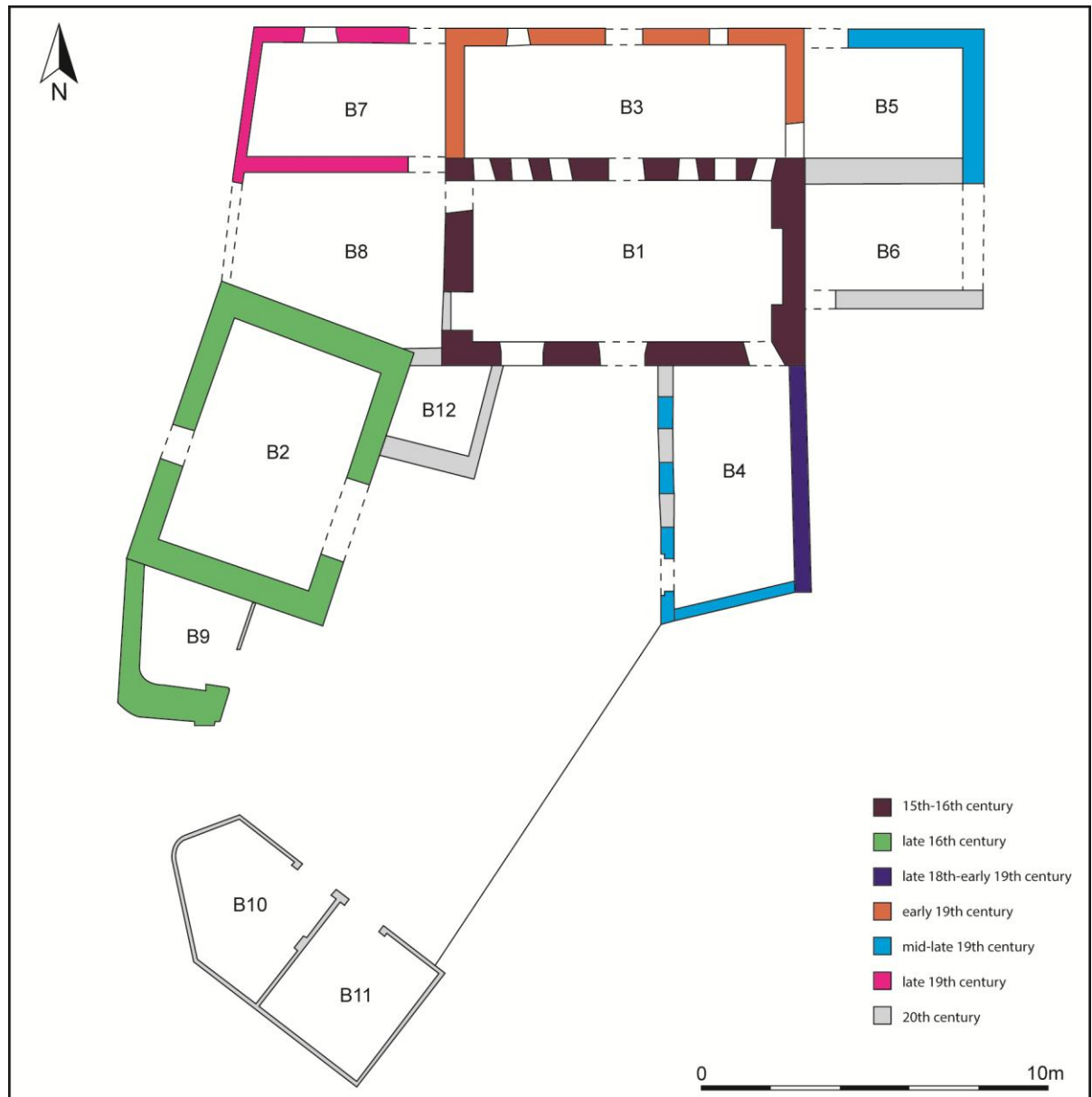
Figure 8: Plan of Higher Velly building complex showing phasing of ground floor wall construction.
