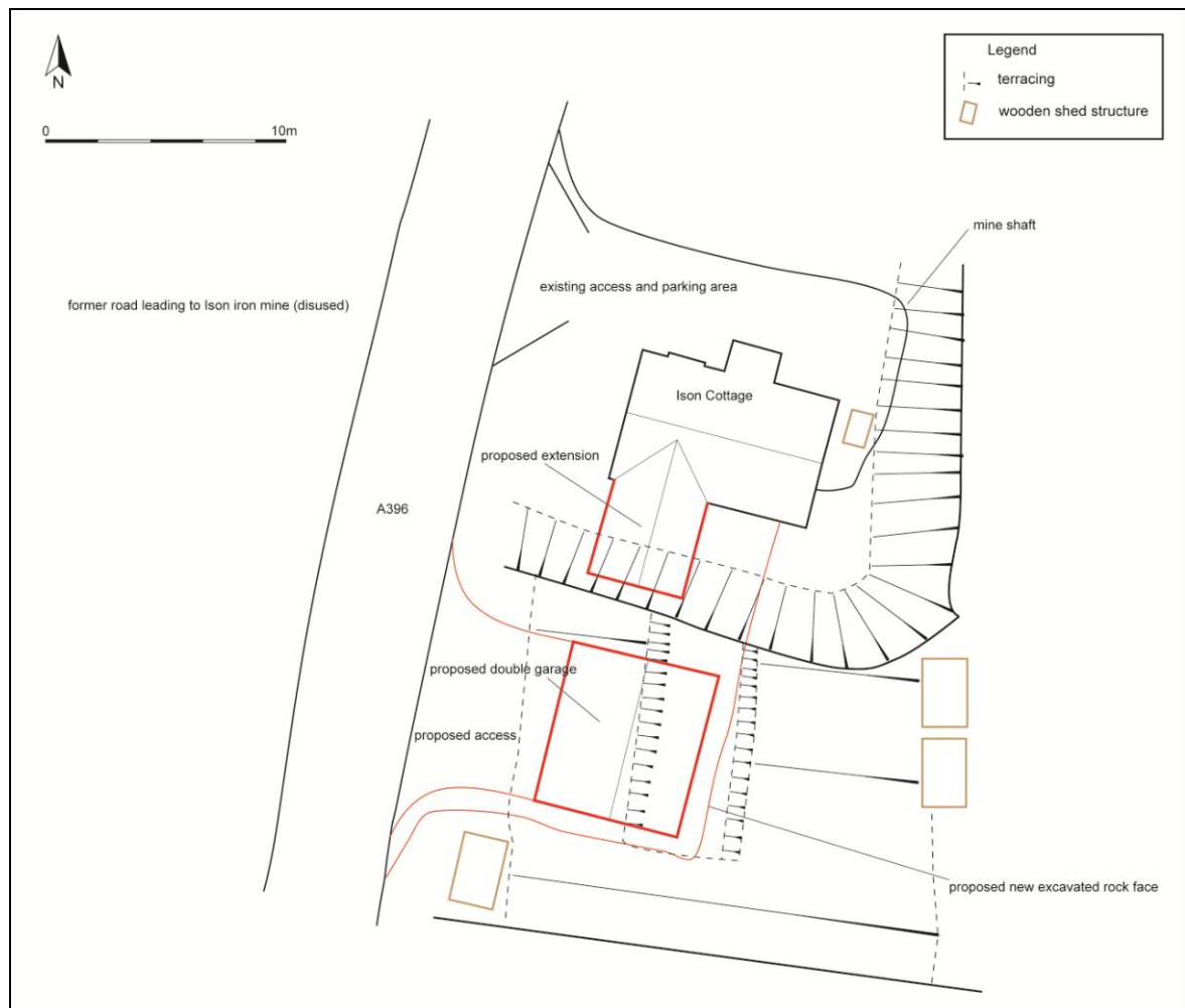
Figure 7: Plan of the site with the footprint of the proposed development shown, with features observed during the walkover survey noted (note this is a measured sketch plan based on the plan provided by the client).
