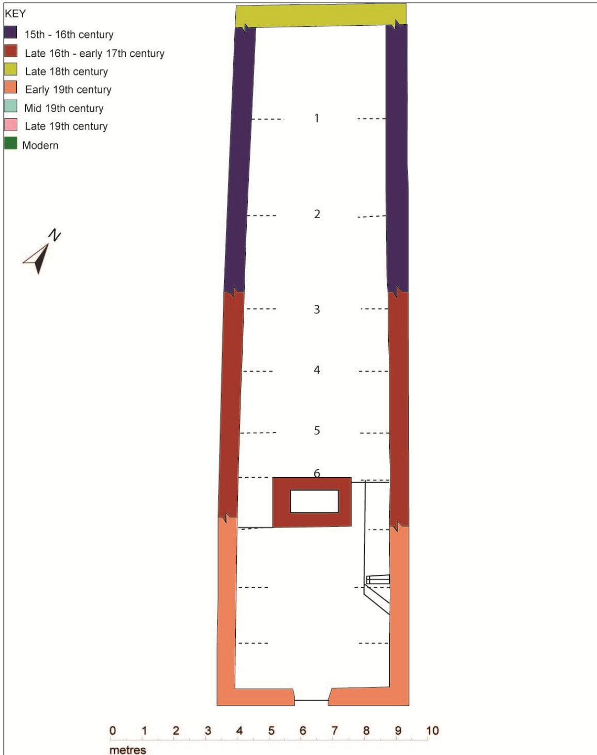
Figure 4: Phased plan attic floor (from the 2015 survey).
