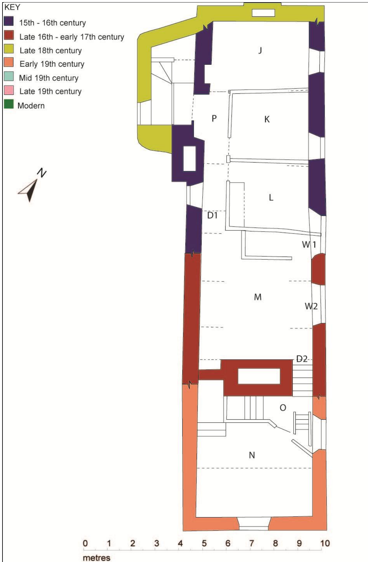
Figure 3: Phased plan first floor (from the 2015 survey).
