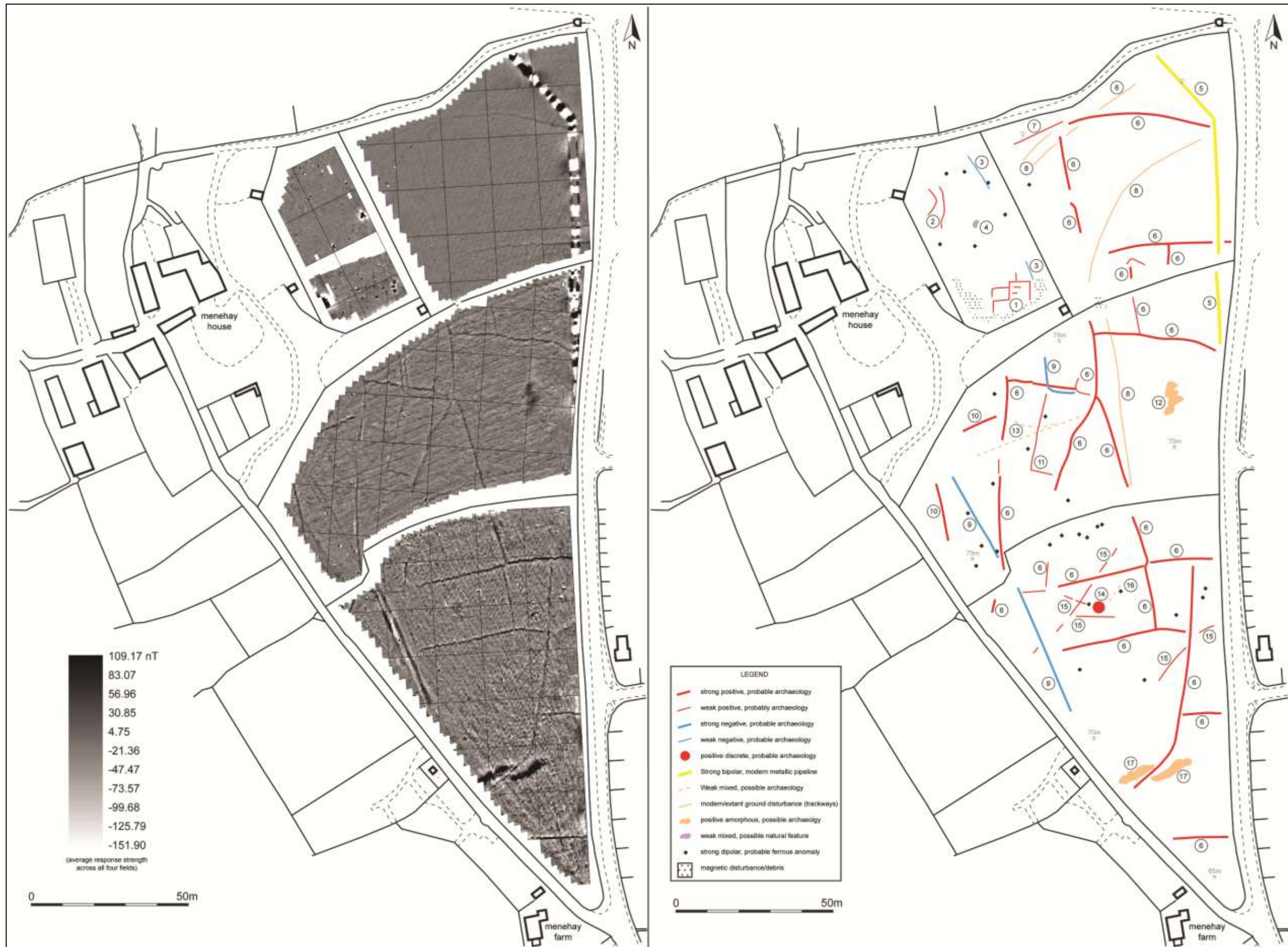
Figure 9: (left) Greyscale shade plot of gradiometer survey data, minimal processing; (right) Interpretation of gradiometer survey data.
