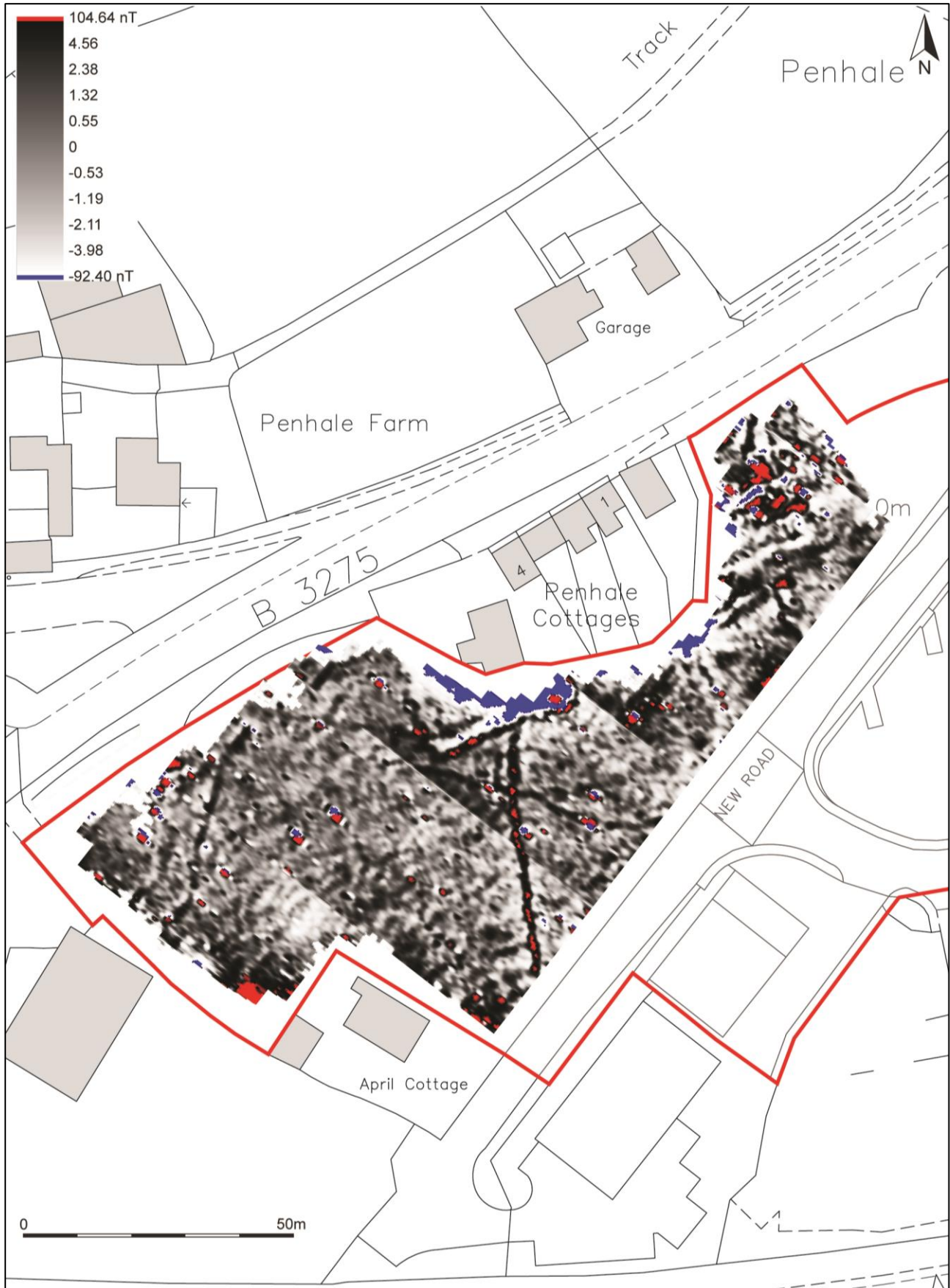
Larger scale red-grey-blue shade plot of gradiometer survey data; band weight equalised, and gradiated shading.
