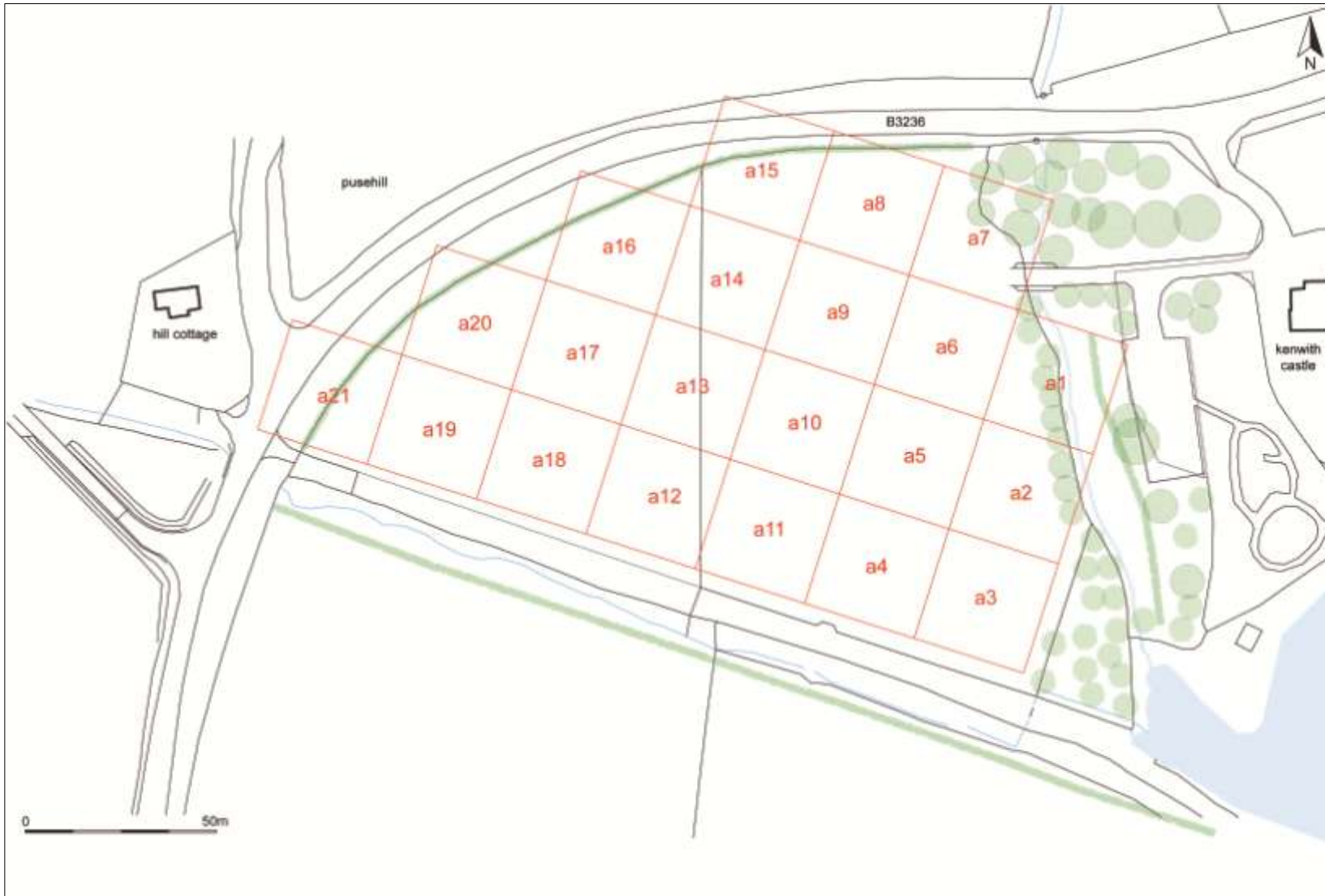
Location and numbering system of geophysical survey grid.
