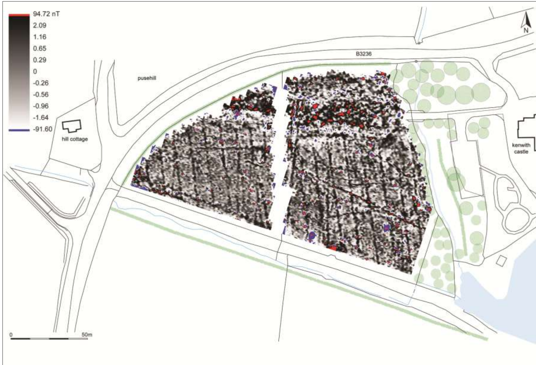
Red-grey-blue shade plot of gradiometer survey data.
