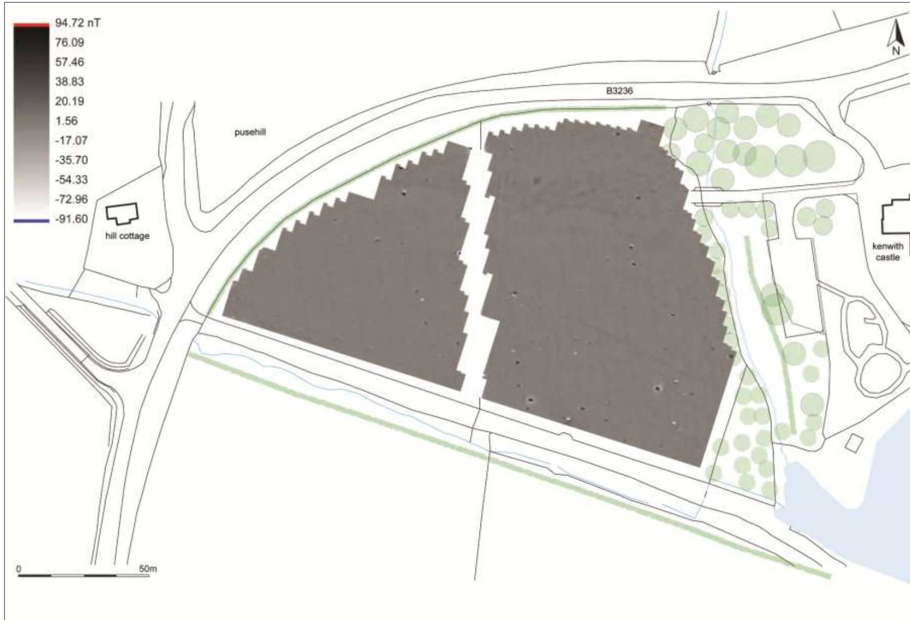
Red-grey-blue shade plot of gradiometer survey data.
