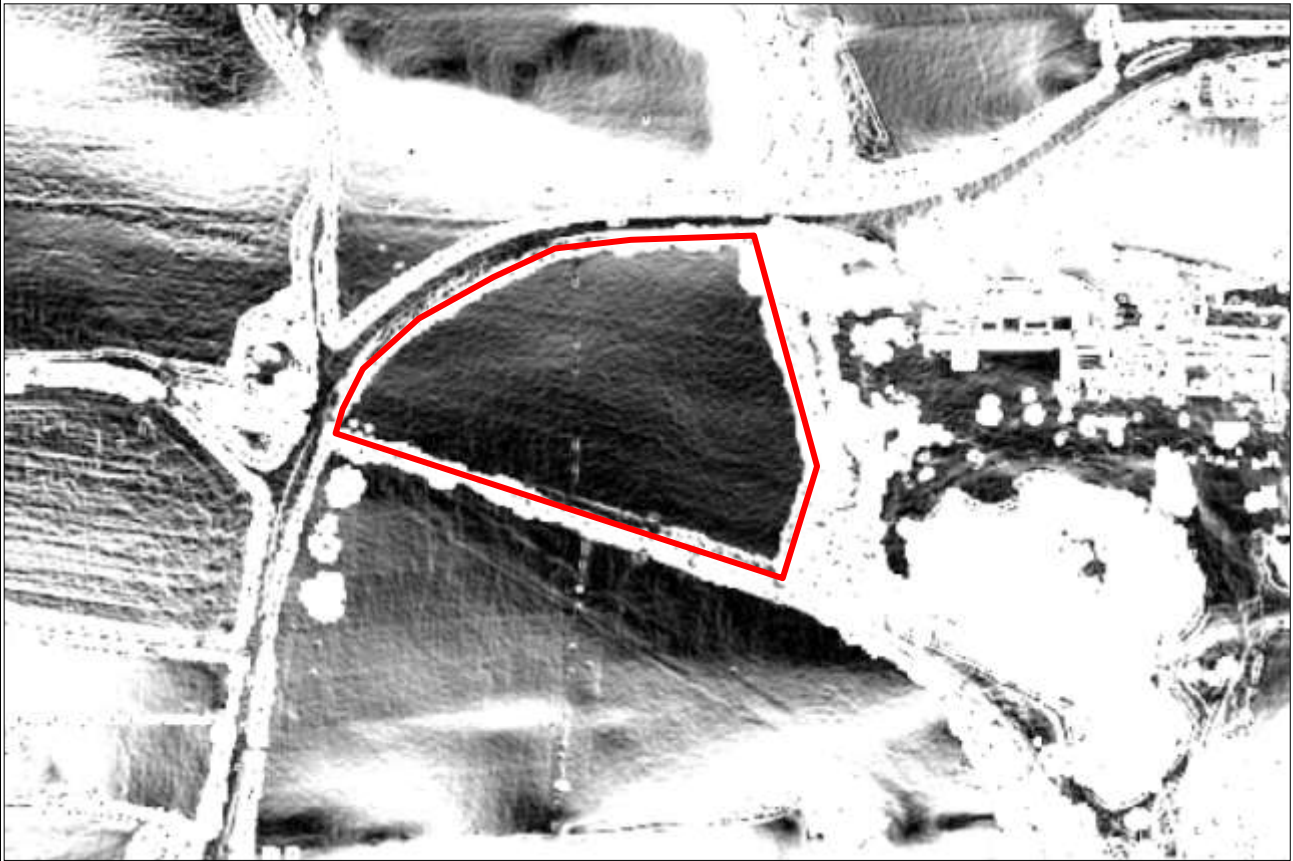
Detailed topographical image based on LiDAR data. This is a QGIS-generated image (terrain analysis>slope) of TELLUS LiDAR survey data [contains freely available LIDAR data supplied by Natural Environment Research Council (Centre for Ecology & Hydrology; British Antarctic Survey; British Geological Survey)]; ©NERC (Centre for Ecology & Hydrology; British Antarctic Survey; British Geological Survey)); the site is indicated in red.
