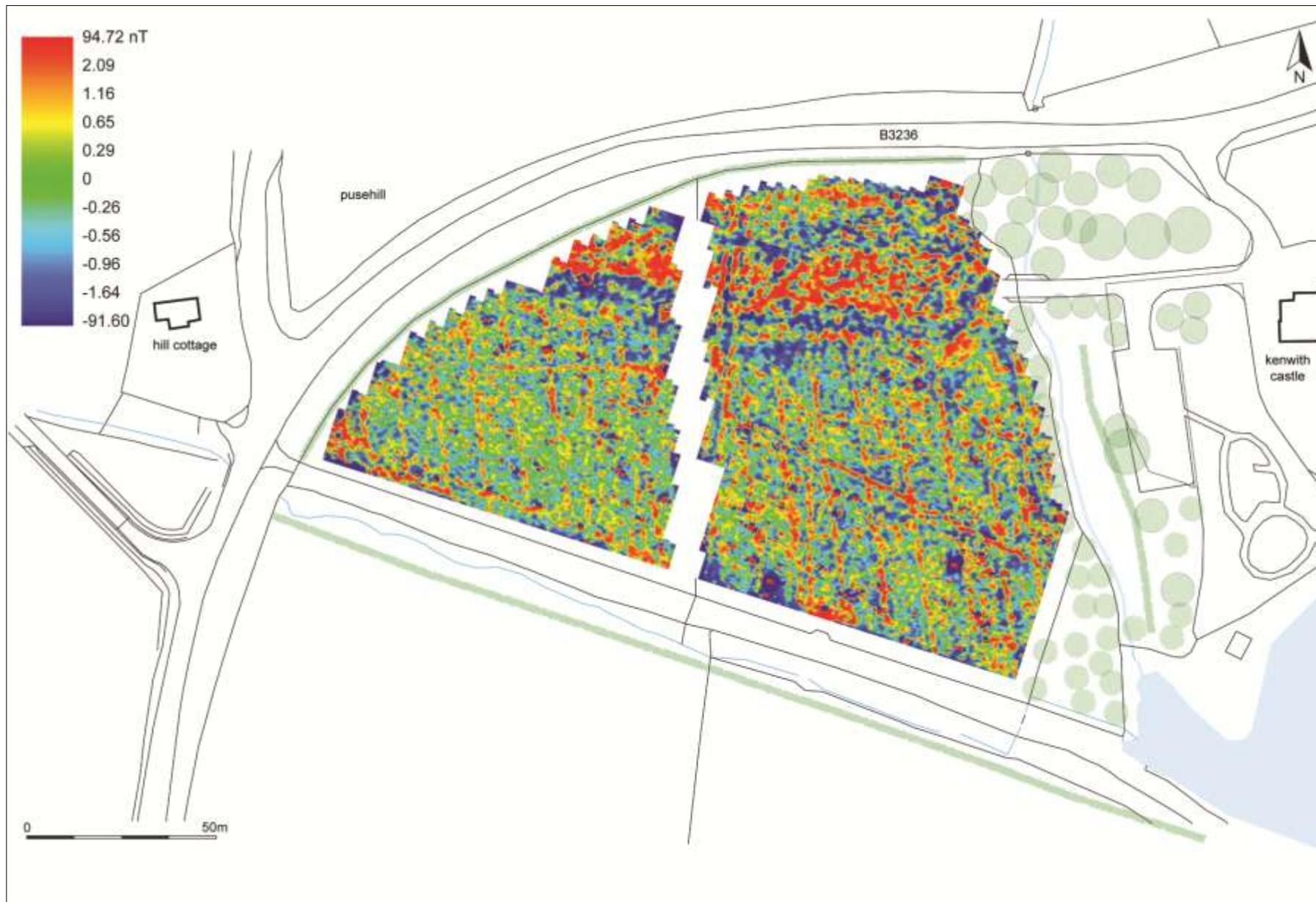
Red-Blue-Green(2) shade plot of gradiometer survey data.
