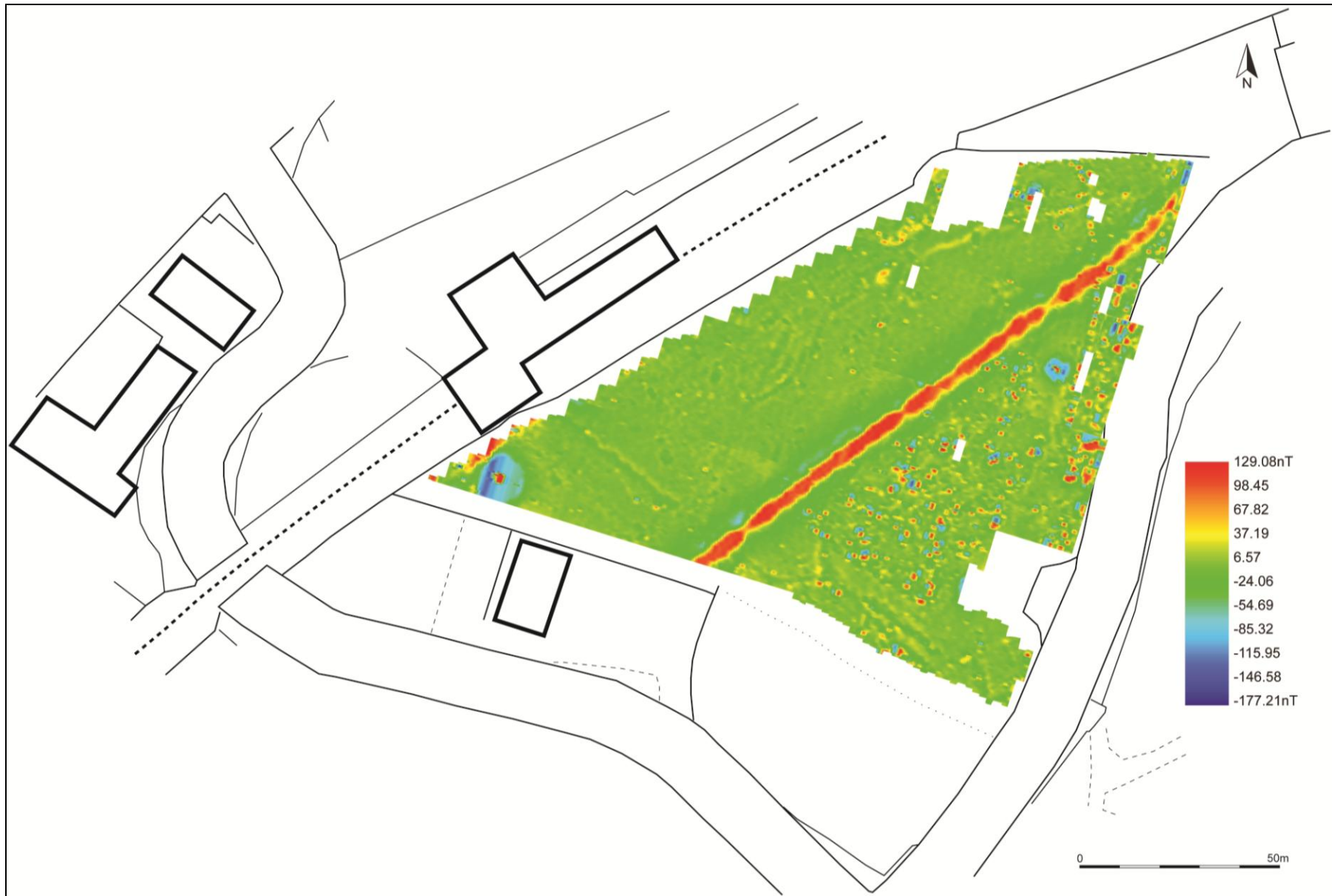
FIGURE 21: RED-BLUE-GREY(2) SHADE PLOT OF GRADIOMETER SURVEY DATA; GRADIATED SHADING.
