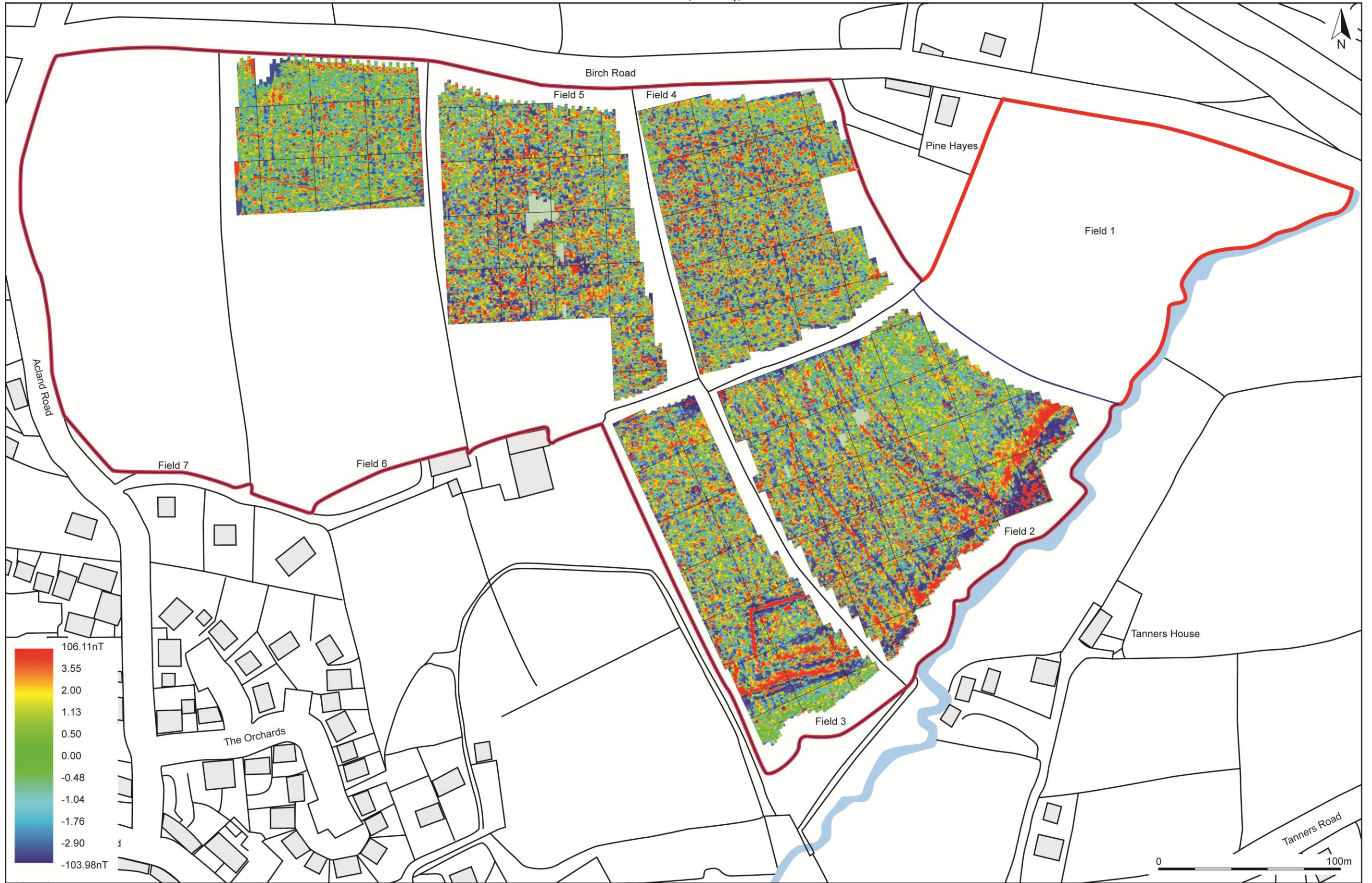
Figure 10: Red-Blue-Green (2) shade plot of gradiometer survey data; gradiated shading.
