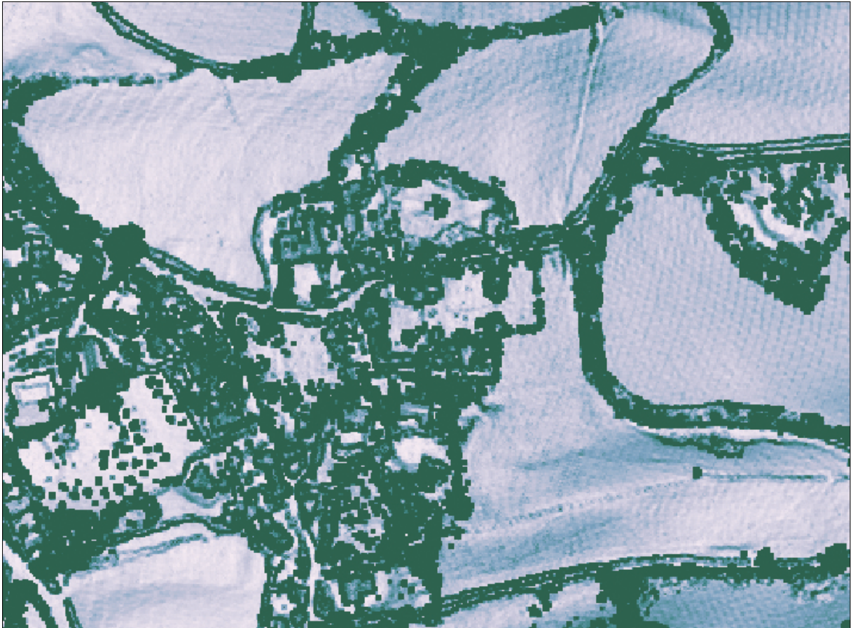
Figure 9: Image using QGIS (terrain analysis: rugged) produced using DSM LiDAR data available from the Environment Agency.
