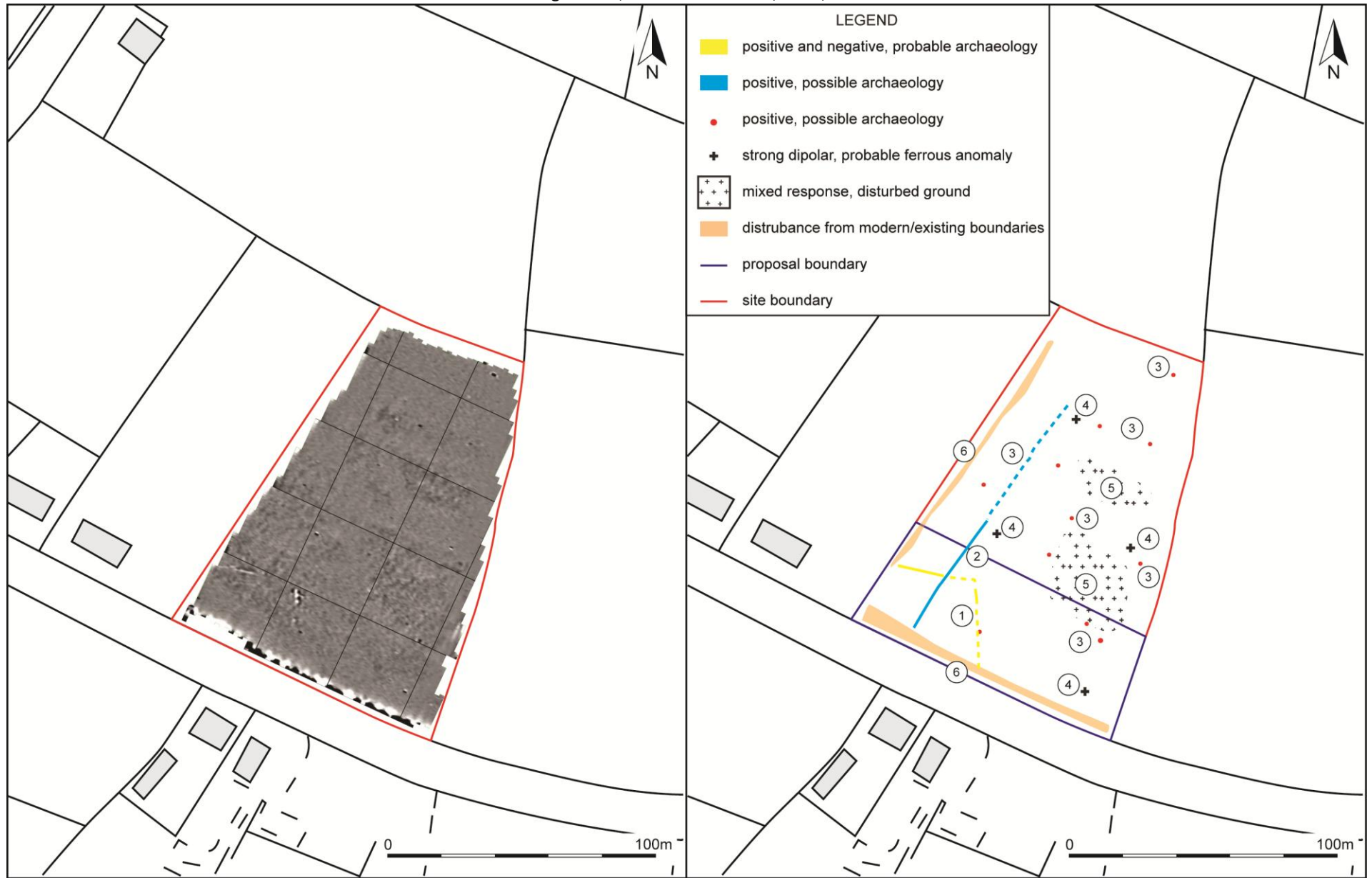
FIGURE 2: SHADE PLOT OF GRADIOMETER SURVEY DATA; MINIMAL PROCESSING (LEFT); INTERPRETATION OF GRADIOMETER SURVEY DATA (RIGHT).
