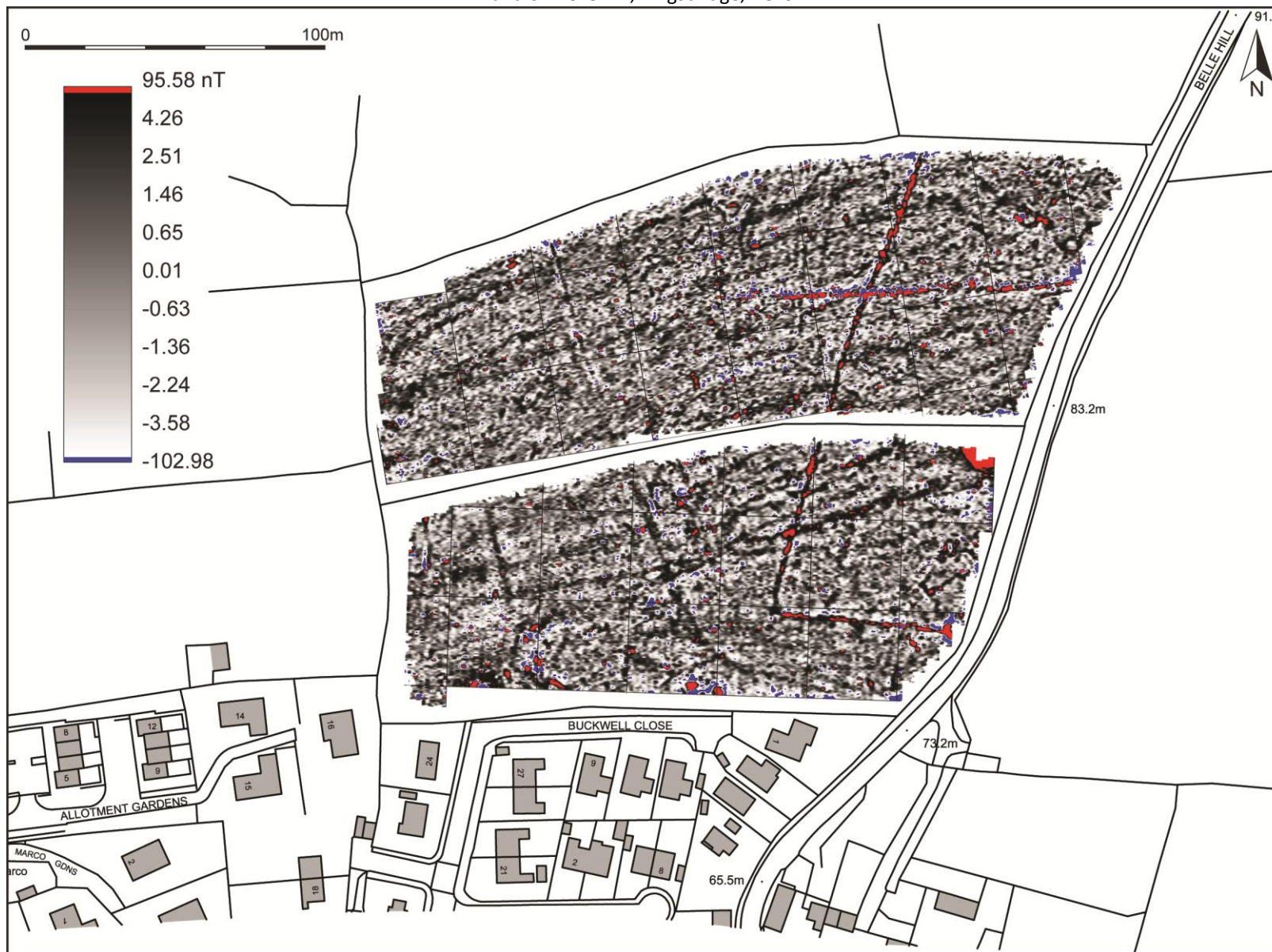
FIGURE 21: RED-GREY-BLUE SHADE PLOT OF GRADIOMETER SURVEY DATA: GRADIATED SHADING; BAND WEIGHT EQUALISED.
