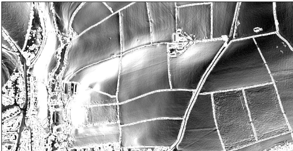
FIGURE 6: DETAILED TOPOGRAPHICAL IMAGE BASED ON LIDAR DATA. THIS IS A QGIS-GENERATED IMAGE (TERRAIN ANALYSIS>SLOPE) OF TELLUS LIDAR SURVEY DATA [CONTAINS FREELY AVAILABLE LIDAR DATA SUPPLIED BY NATURAL ENVIRONMENT RESEARCH COUNCIL (CENTRE FOR ECOLOGY & HYDROLOGY; BRITISH ANTARCTIC SURVEY; BRITISH GEOLOGICAL SURVEY); ©NERC (CENTRE FOR ECOLOGY & HYDROLOGY; BRITISH ANTARCTIC SURVEY; BRITISH GEOLOGICAL SURVEY)].
