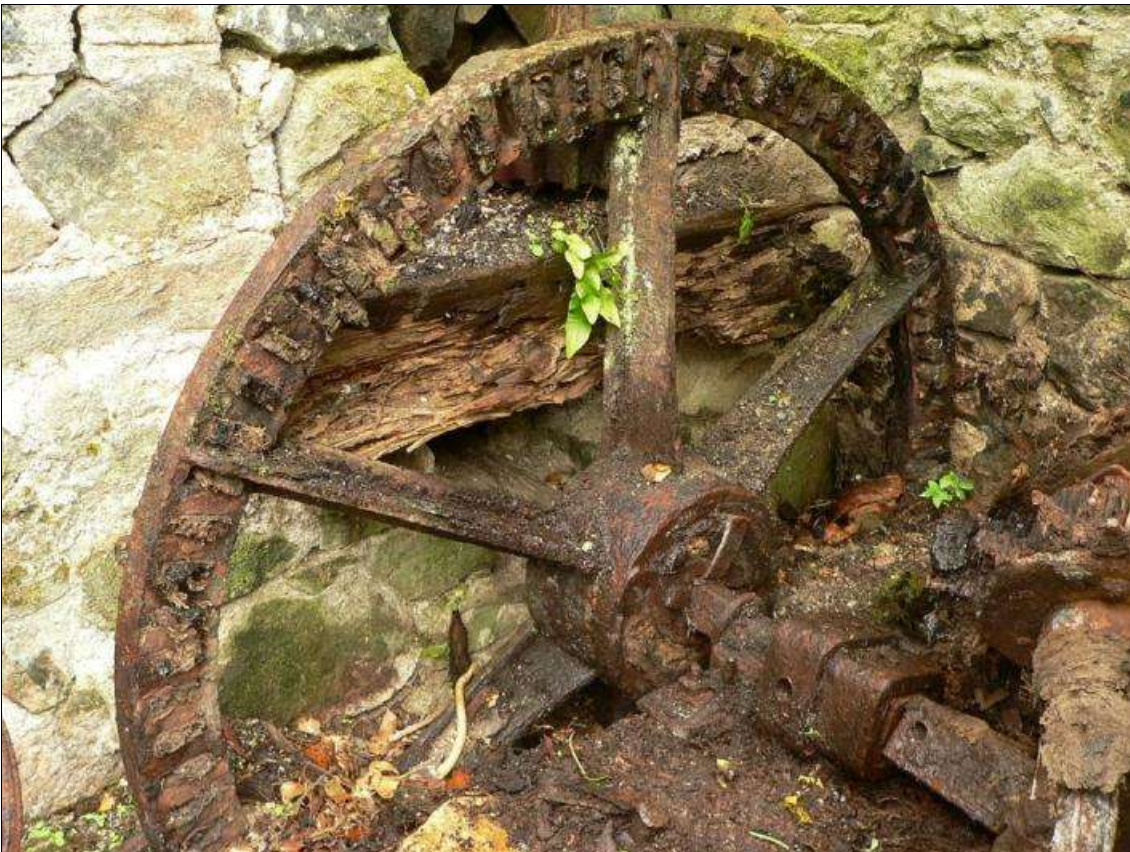
Bevel gear on western extension of layshaft, for driving vertical spindle (photo: M Watts).
