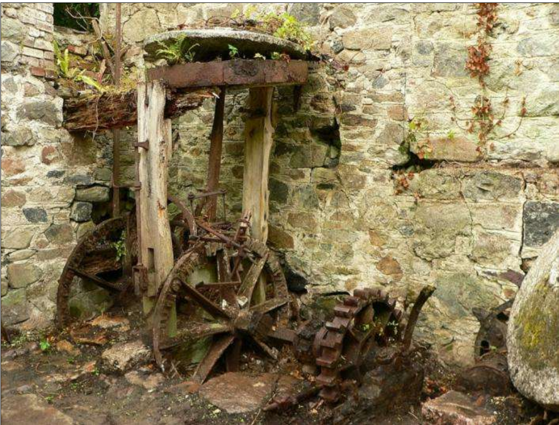
Upstream layshaft, driving gears and millstones, looking north-west (photo: M Watts).
