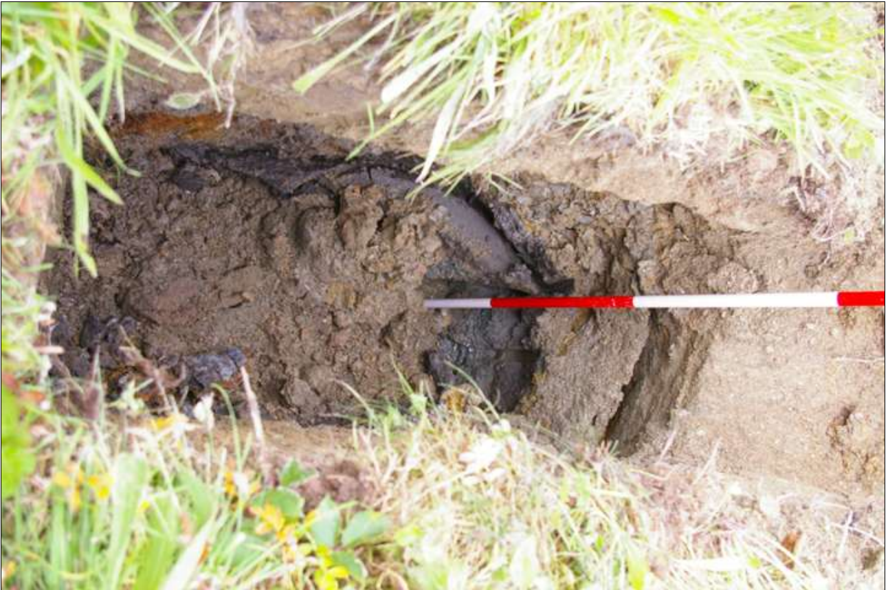
Geotechnical pit #2, viewed from the south (scale 2m); note the dark grey humic silty-clay in the partly-collapsed pit.
