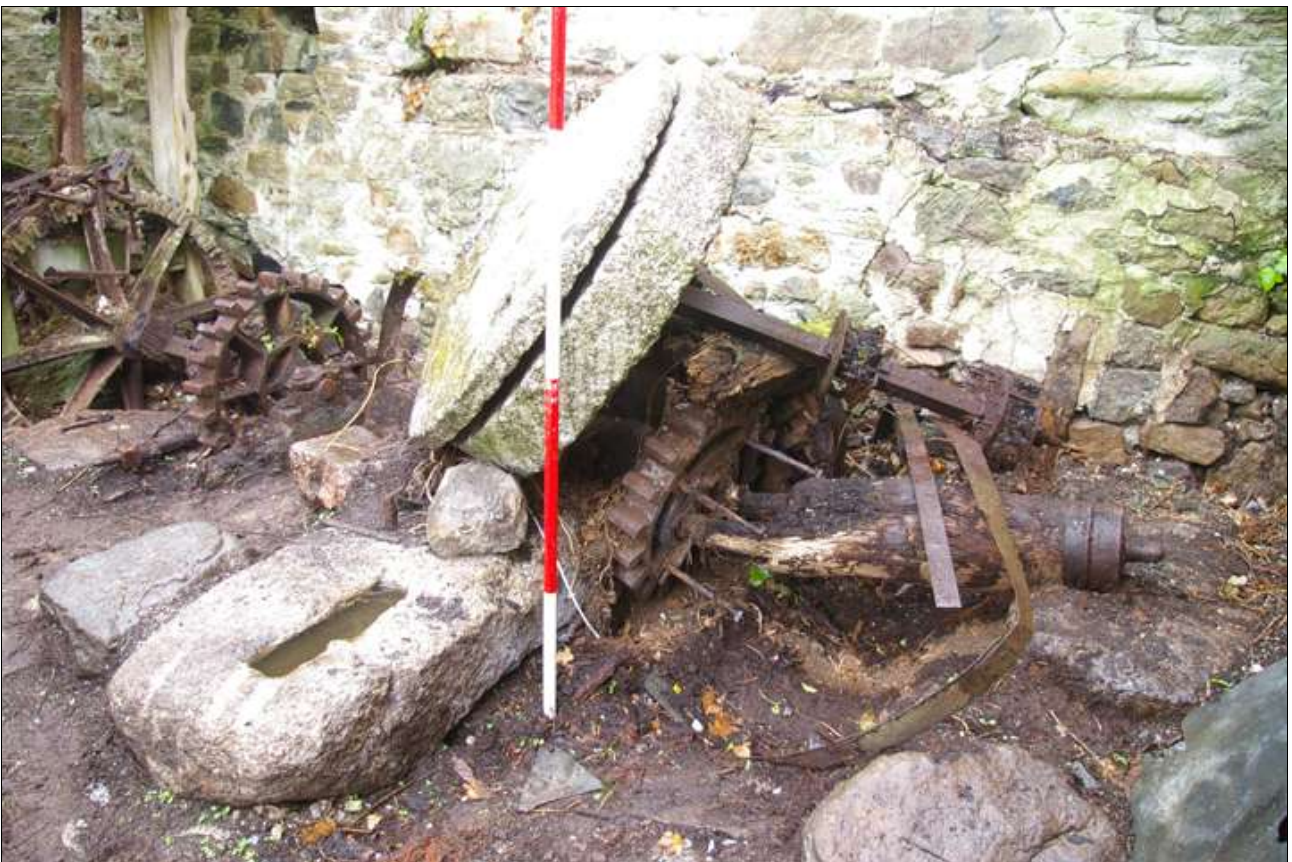
The collapsed downstream iron spur gear and millstones; viewed from the south-east (scale 2m).
