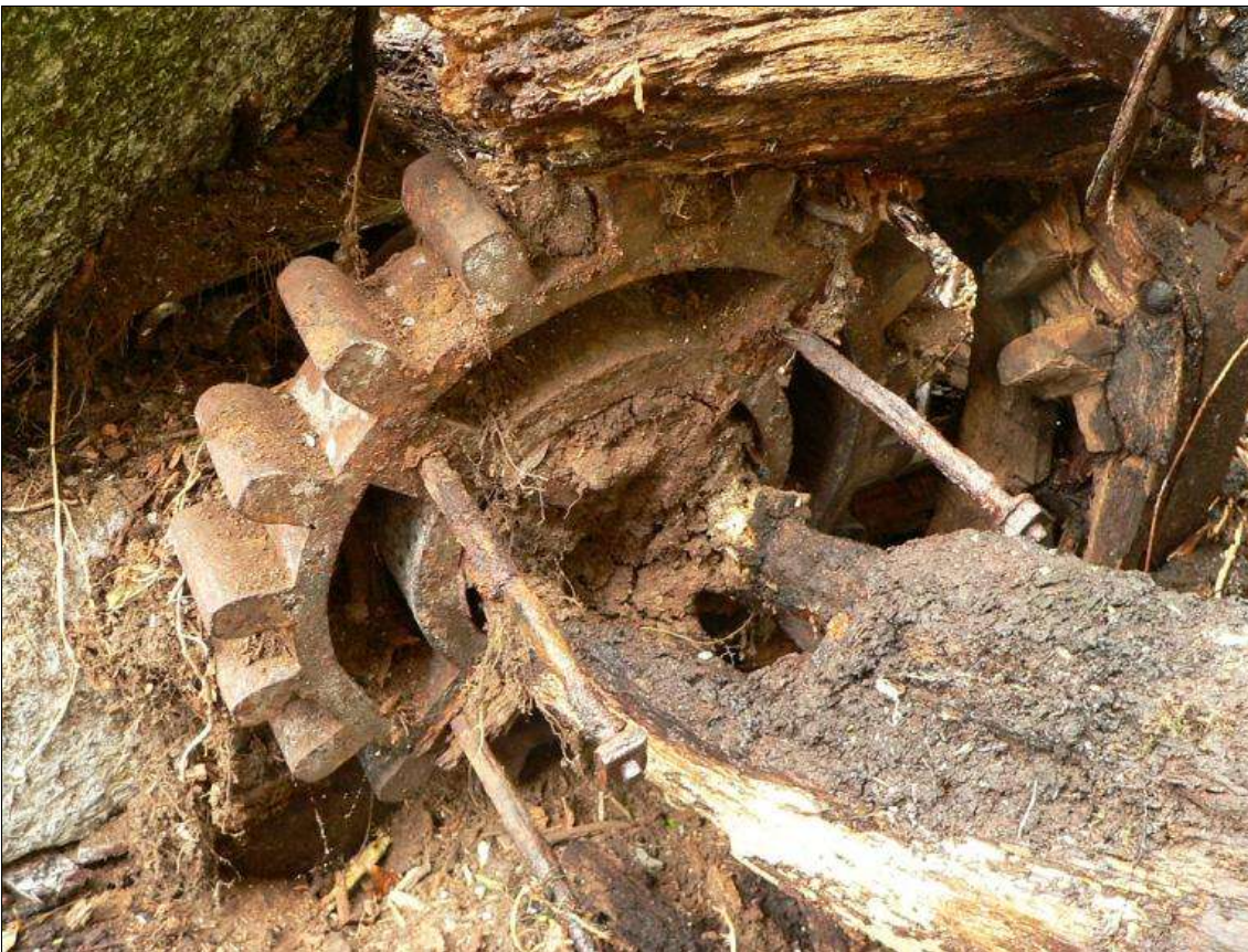
Remains of downstream layshaft, with iron spur pinion (driven by pitwheel) and bolts for securing it to arms of stone drive gear (rotted away) (photo: M Watts).
