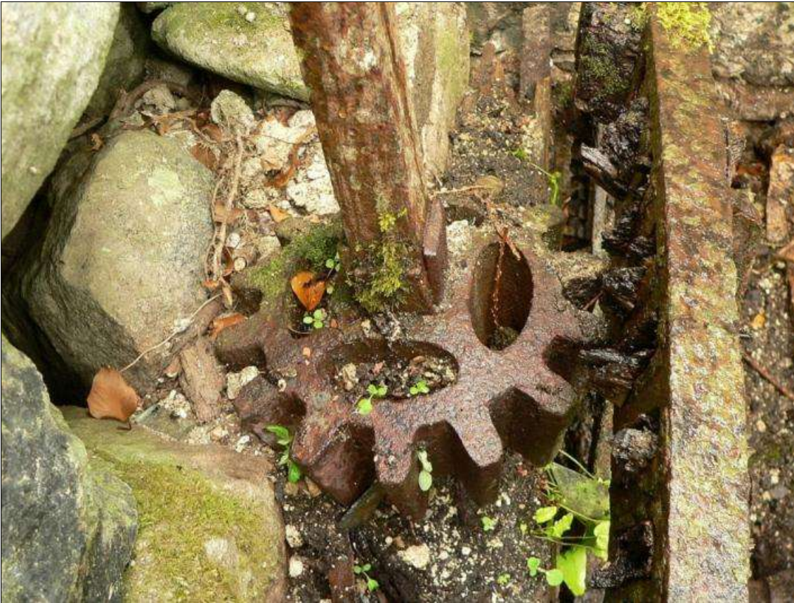
Pinion on foot of vertical spindle (photo: M Watts).
