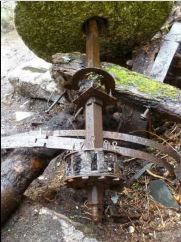
LEFT: Stone spindle to downstream millstones with remains of stone nut and jigger drive pulley. The two iron bands bound the circumference of the timber/stone drive wheel (photo: M Watts). RIGHT: Collapsed remains of waterwheel (photo: M Watts).
