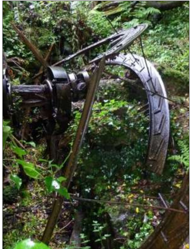
LEFT: Stone spindle to downstream millstones with remains of stone nut and jigger drive pulley. The two iron bands bound the circumference of the timber/stone drive wheel (photo: M Watts). RIGHT: Collapsed remains of waterwheel (photo: M Watts).
