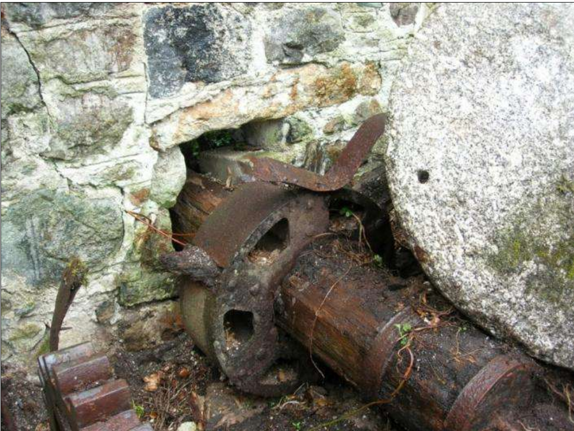
Pitwheel centre and inner end of waterwheel shaft (photo: M Watts).
