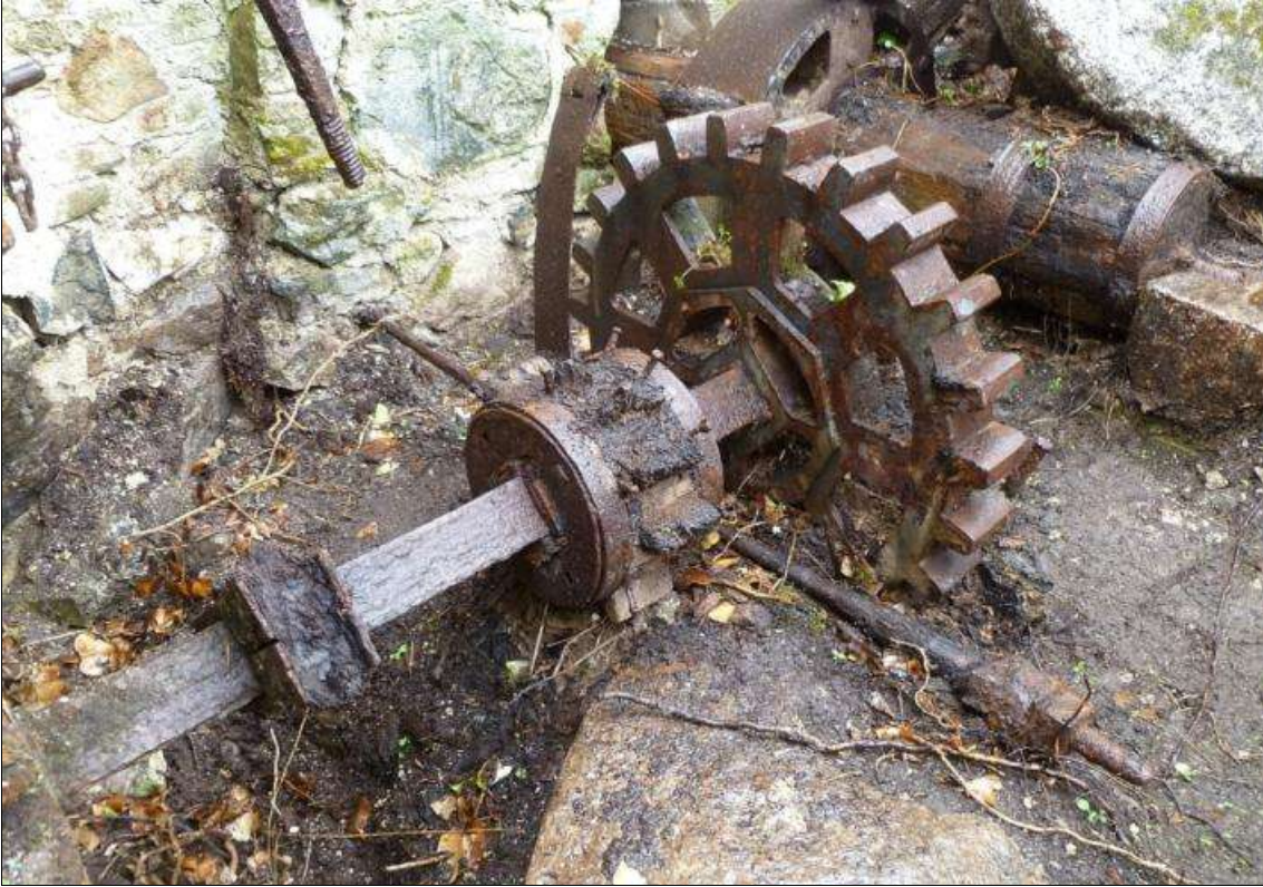
Spur pinion driven from pitwheel and east end of upstream layshaft (photo: M Watts).
