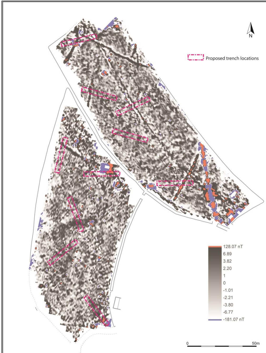
Figure 15: Plan of the proposed trench locations, shown on a plot of the geophysical survey results.
