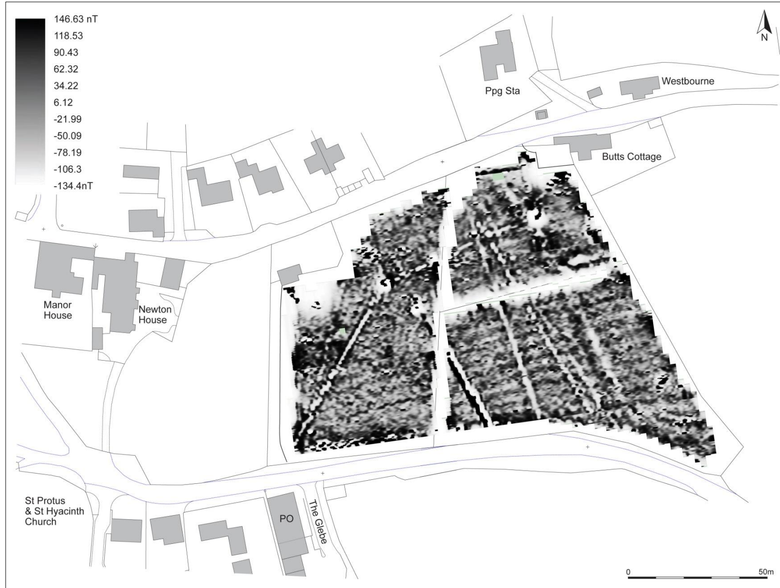
Greyscale shade plot of gradiometer survey data; Band Weight Equalised, Gradiated Shading.
