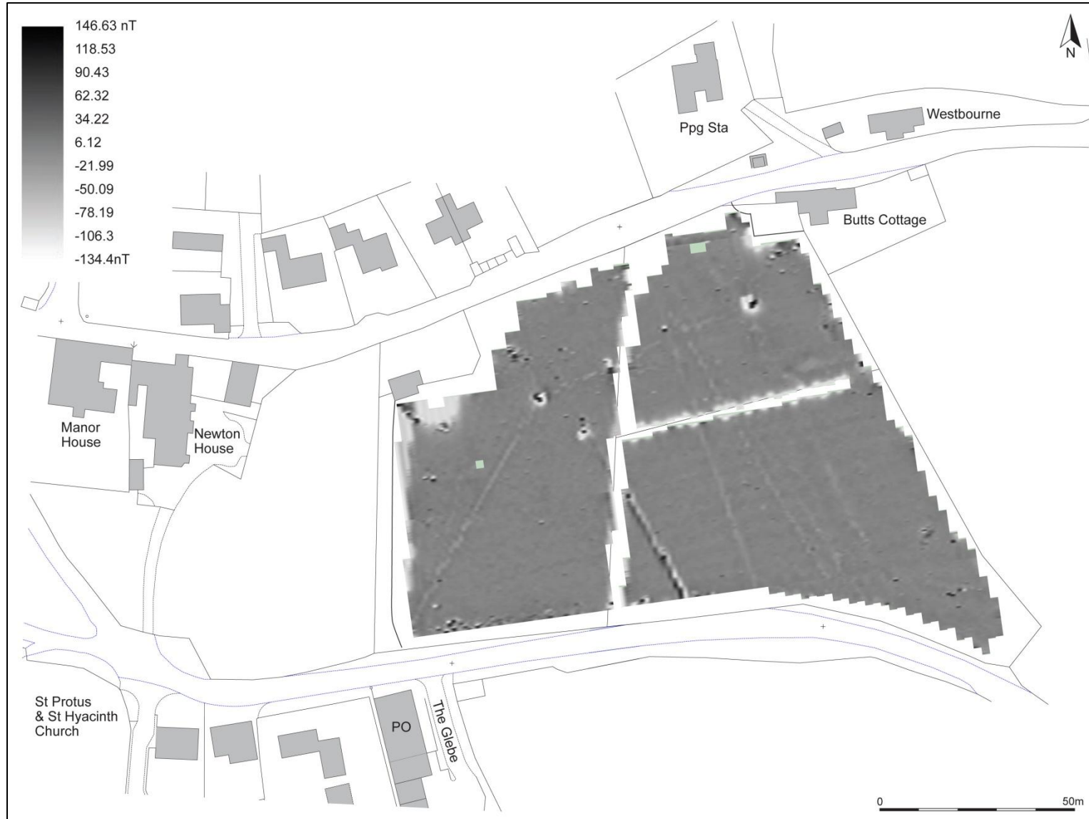
Greyscale shade plot of gradiometer survey data; Gradiated Shading.
