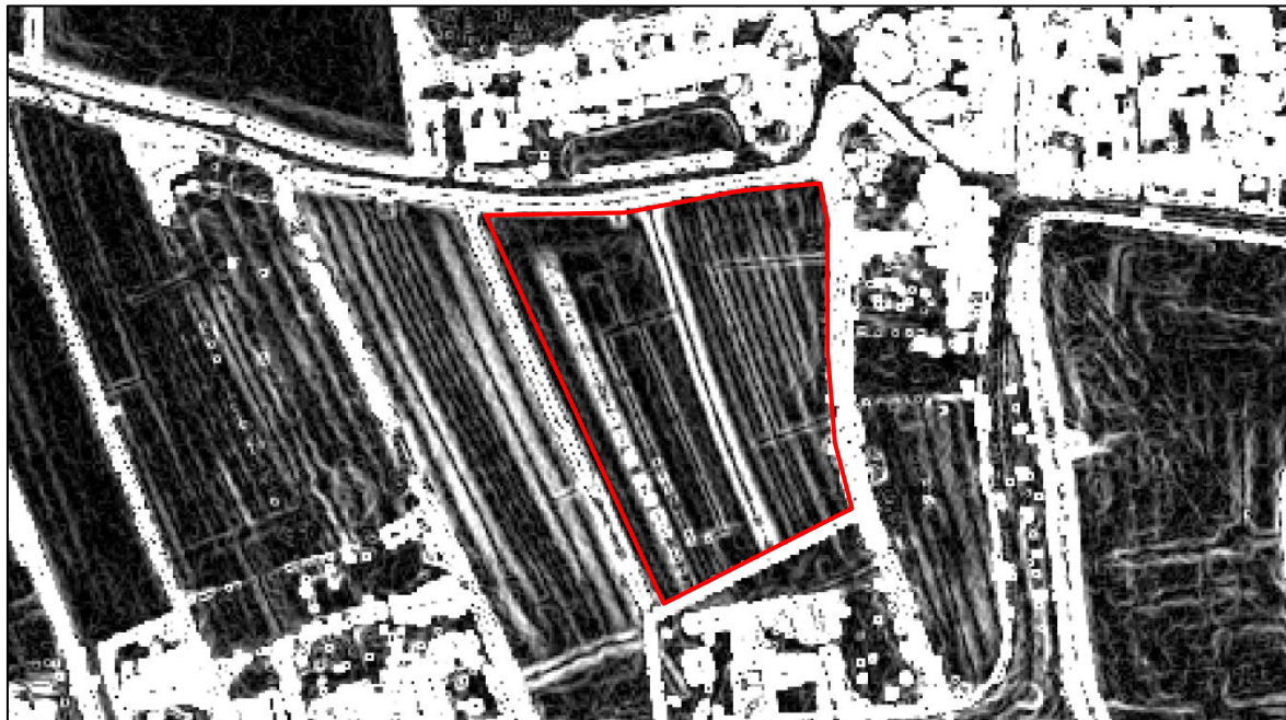
Figure 5: Detailed topographical image based on LiDAR data. This is a QGIS-generated image (terrain analysis>slope) of TELLUS LiDAR survey data [contains freely available LIDAR data supplied by Natural Environment Research Council (Centre for Ecology & Hydrology; British Antarctic Survey; British Geological Survey); ©NERC (Centre for Ecology & Hydrology; British Antarctic Survey; British Geological Survey)]; the site is outlined in red.
