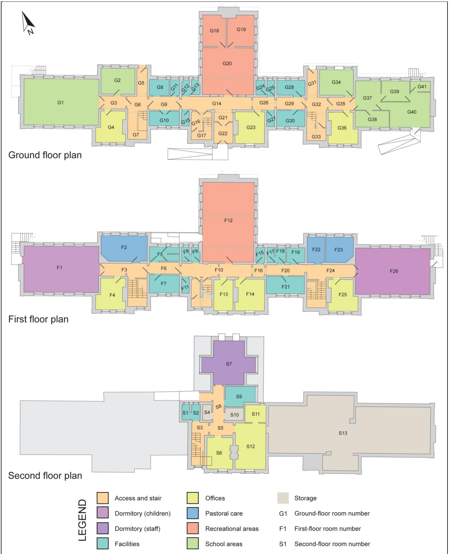
FIGURE 10: BUILDING PLANS SHOWING INTENDED ROOM FUNCTION.
