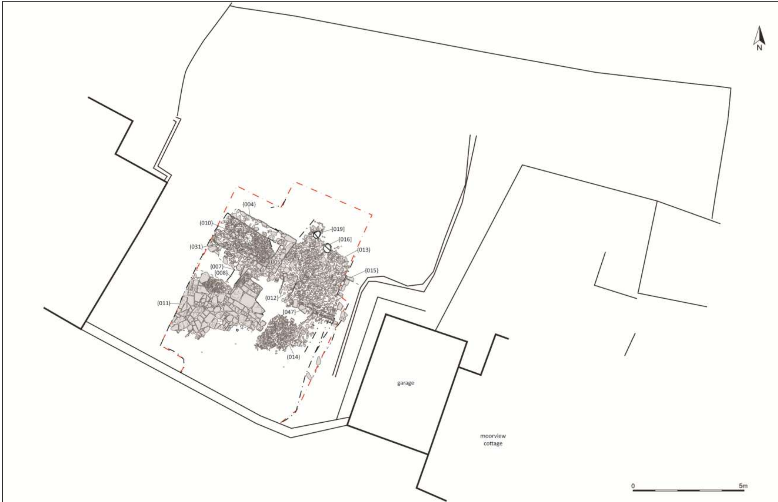
FIGURE 4: SITE PLAN: PHASE 3 POST-MEDIEVAL FLOORS (010), (011), (013) AND (014); POSTHOLES [016] AND [019]; AND WALLS {004}, {005}, {006}, {007} AND {012} OF A STRUCTURE.
