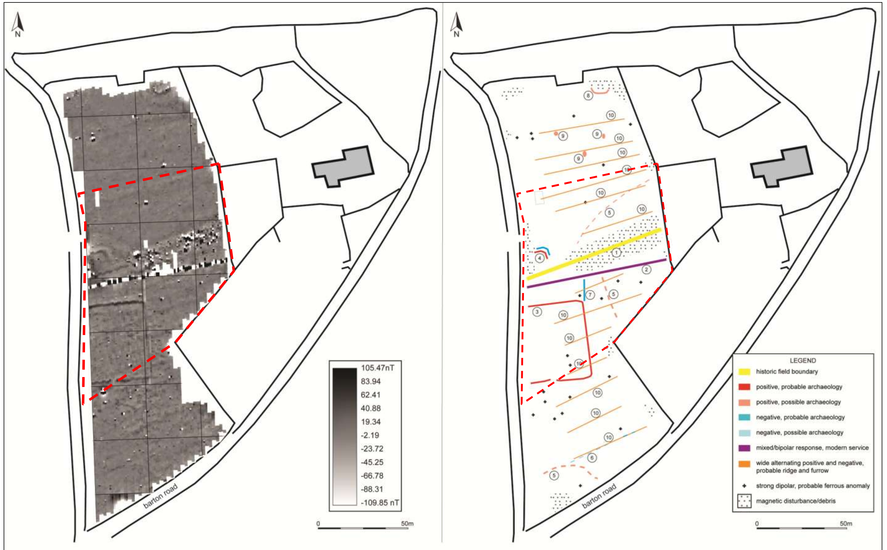
FIGURE 7: (LEFT) SHADE PLOT OF GRADIOMETER SURVEY DATA, MINIMAL PROCESSING; (RIGHT) INTERPRETATION OF GRADIOMETER SURVEY DATA. THE PROPOSAL SITE IS BOUNDED BY RED DASHED LINES.
