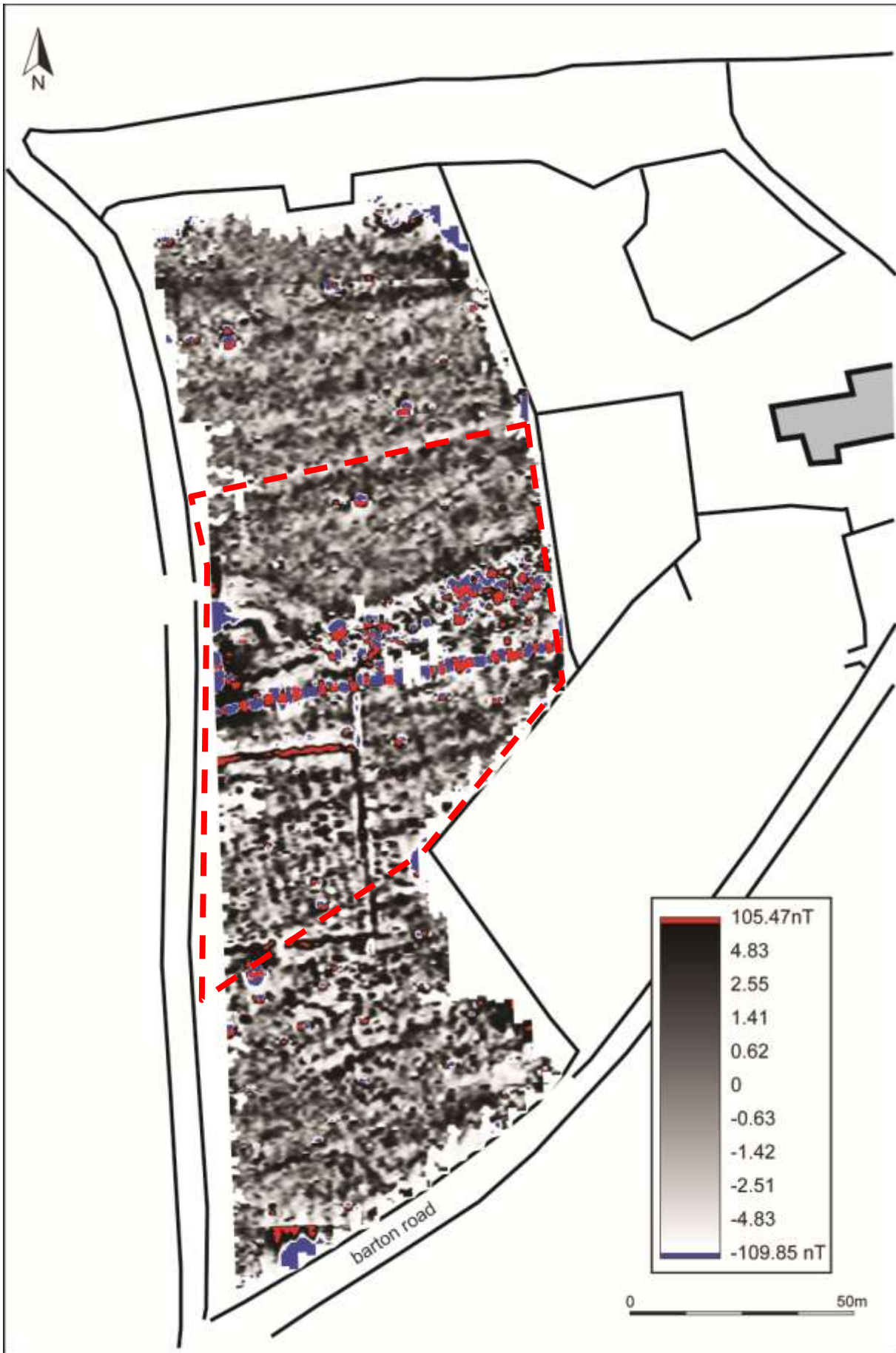
RED-GREY-BLUE SHADE PLOT OF GRADIOMETER SURVEY DATA; GRADIATED SHADING; BAND WEIGHT EQUALISED.
