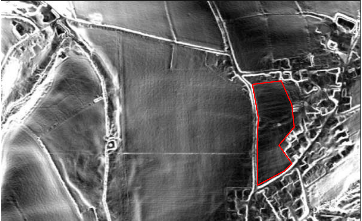
FIGURE 10: DETAILED TOPOGRAPHICAL IMAGE BASED ON LIDAR DATA. THIS IS A QGIS-GENERATED IMAGE (TERRAIN ANALYSIS>SLOPE) OF ENVIRONMENT AGENCY LIDAR SURVEY DATA [CONTAINS FREELY AVAILABLE LIDAR DATA SUPPLIED BY NATURAL ENVIRONMENT RESEARCH COUNCIL (CENTRE FOR ECOLOGY & HYDROLOGY; BRITISH ANTARCTIC SURVEY; BRITISH GEOLOGICAL SURVEY); ©NERC (CENTRE FOR ECOLOGY & HYDROLOGY; BRITISH ANTARCTIC SURVEY; BRITISH GEOLOGICAL SURVEY)].
