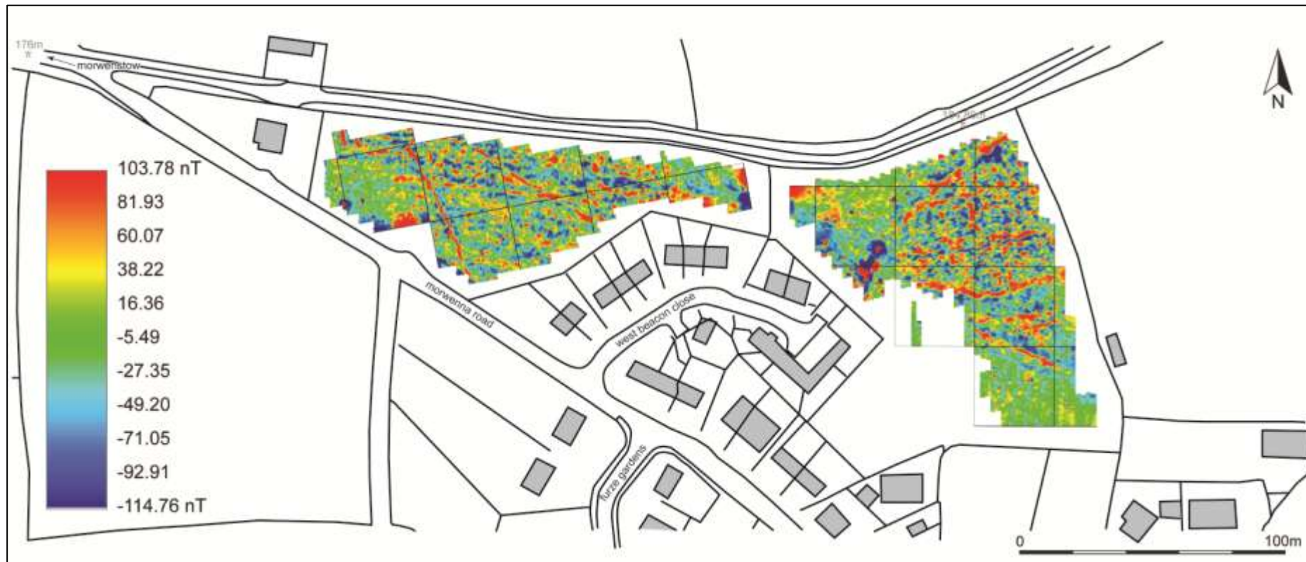
FIGURE 16: RED-BLUE-GREY (2) SHADE PLOT OF GRADIOMETER SURVEY DATA: GRADIATED SHADING; BAND WEIGHT EQUALISED.
