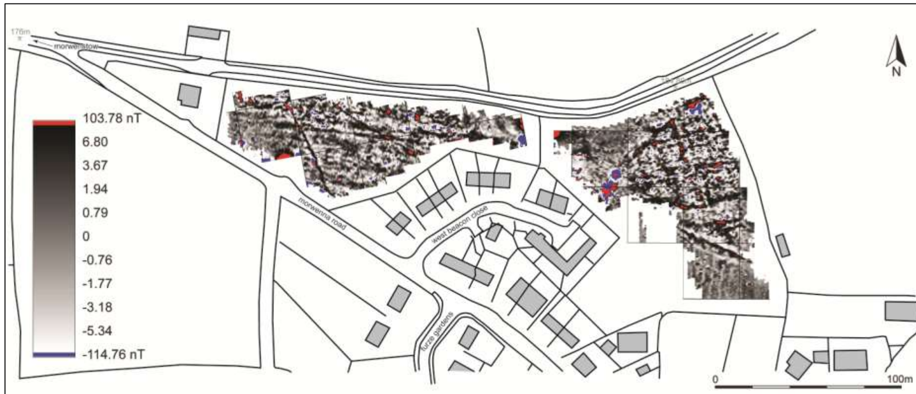
FIGURE 15: RED-GREY-BLUE SHADE PLOT OF GRADIOMETER SURVEY DATA: GRADIATED SHADING; BAND WEIGHT EQUALISED.
