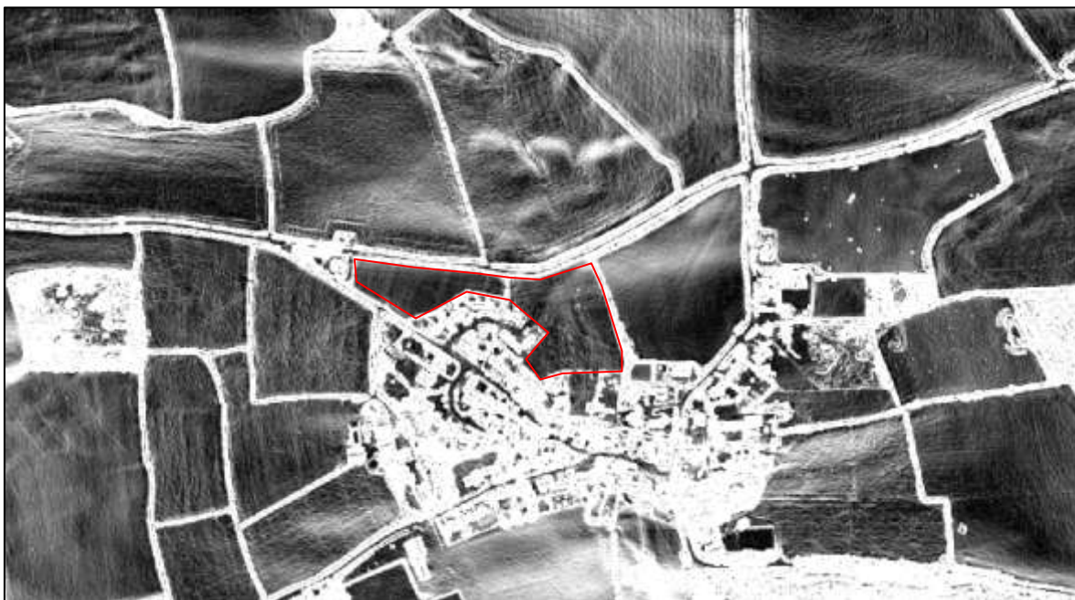
Figure 7: Detailed topographical image based on LiDAR data. This is a QGIS-generated image (terrain analysis>slope) of TELLUS LiDAR survey data [contains freely available LIDAR data supplied by Natural Environment Research Council (Centre for Ecology & Hydrology; British Antarctic Survey; British Geological Survey); ©NERC (Centre for Ecology & Hydrology; British Antarctic Survey; British Geological Survey)]; the site is outlined in red.
