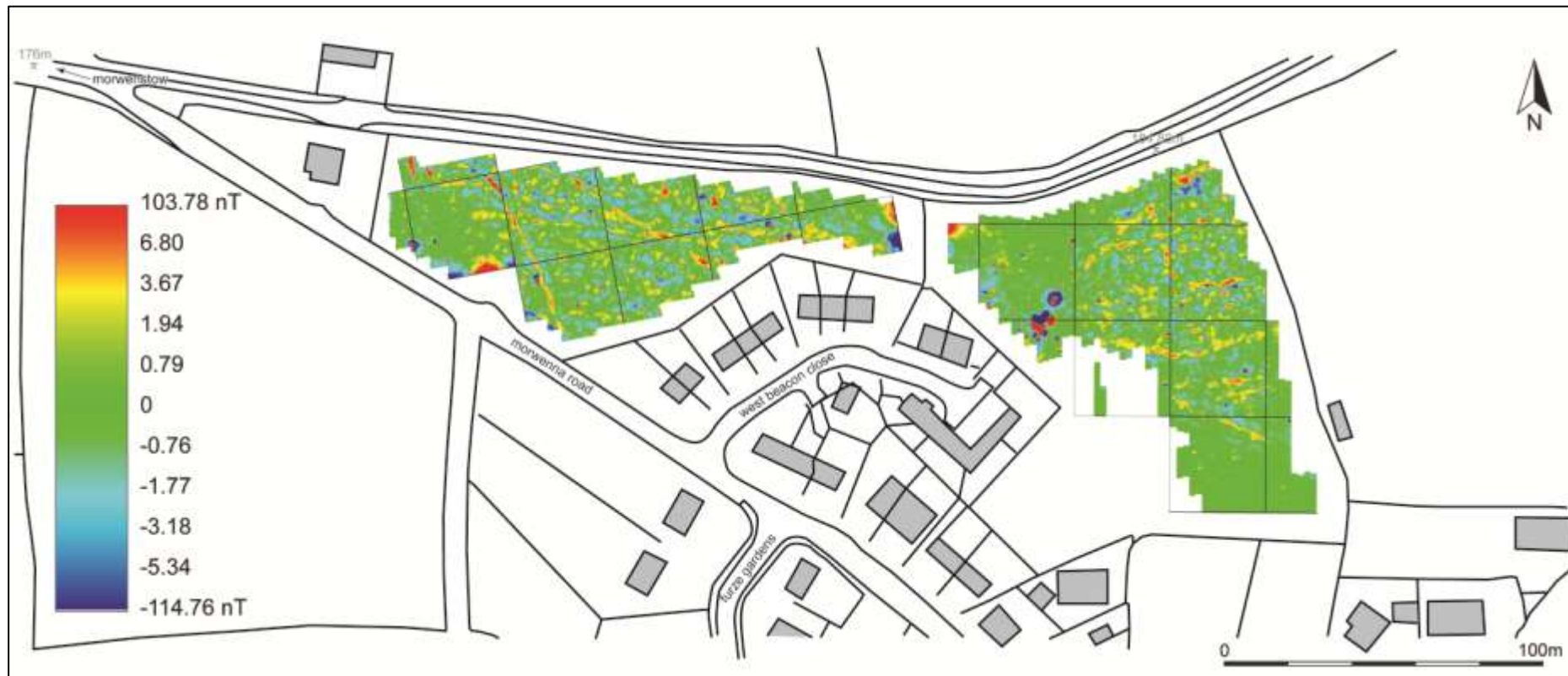
FIGURE 17: RED-BLUE-GREY (1) SHADE PLOT OF GRADIOMETER SURVEY DATA: GRADIATED SHADING.
